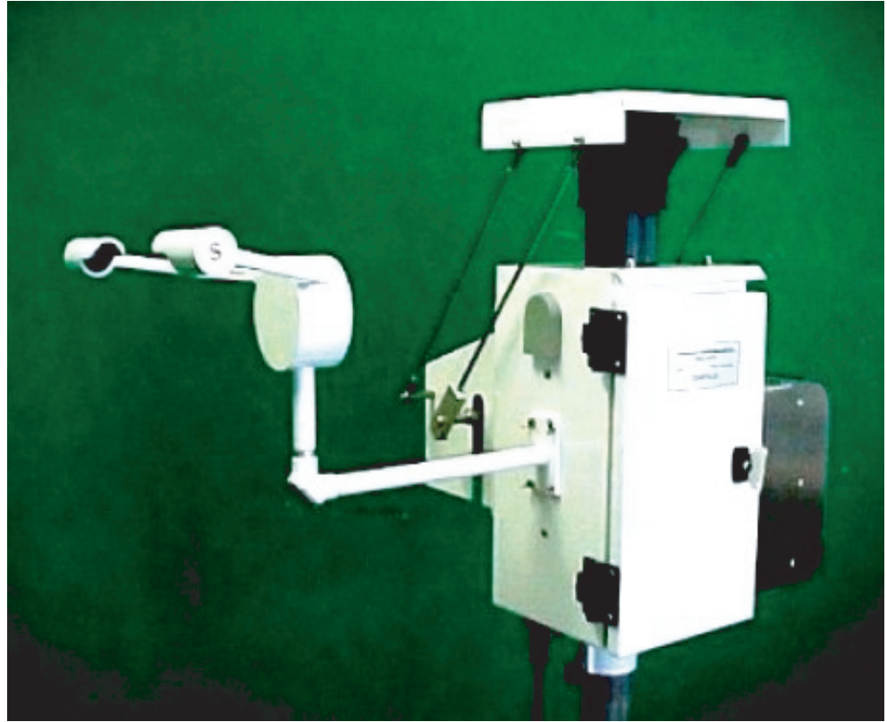
Figure 3. Photograph showing the National Atmospheric Deposition Program/Mercury Deposition Network precipitation collector manufactured by N-CON Systems (N-CON Systems Co., Inc., 2004).
