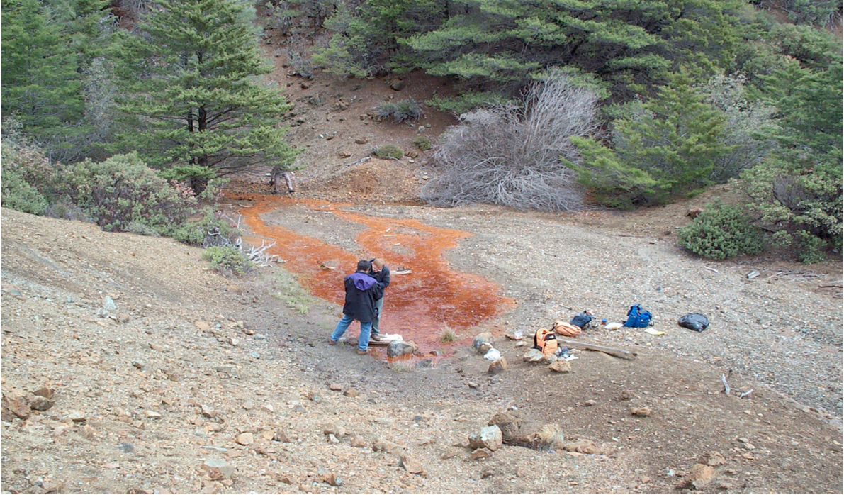
Figure 9. Lower mine drainage seep at Helen Mine at the base of the waste-rock pile sampled in April during the wet season (sample site 21HM2).
