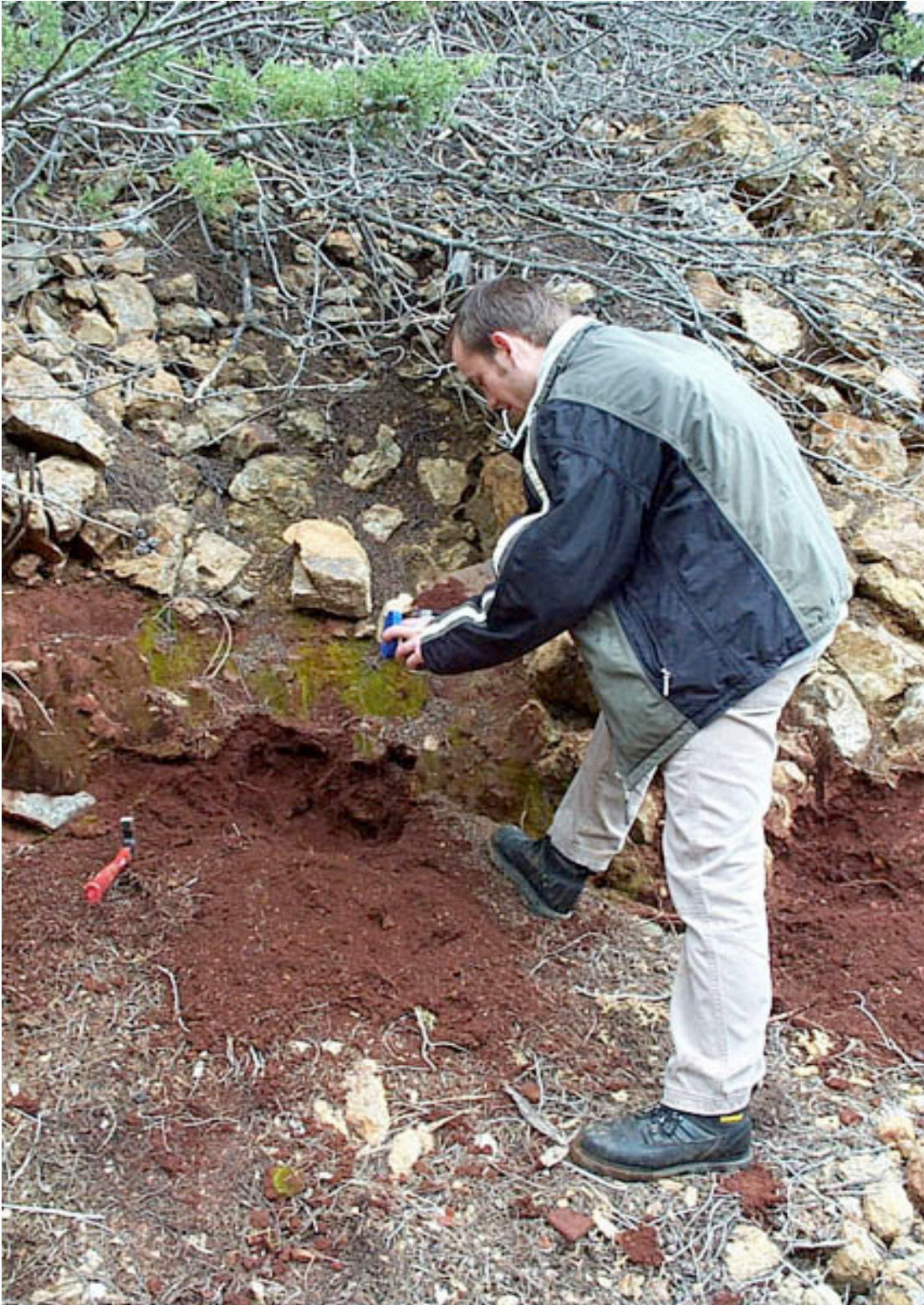
Figure 18. Calcines and condenser soot (sample sites 21-CH-4C, 450 ppm Hg,) below waste rock near ore crib (lower right in fig. 15) in north bank of Dry Creek at Chicago Mine area.
