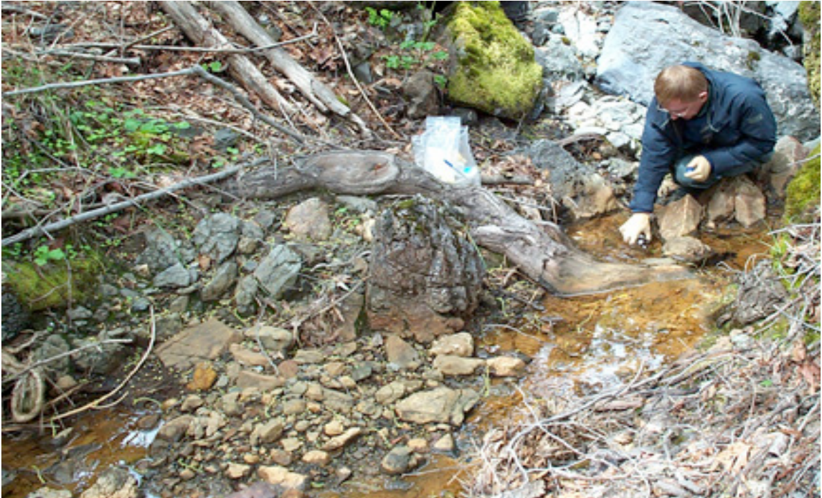
Figure 10. Helen tributary coated with \text{FeOOH} resulting from mine drainage from the Helen Mine area. The site is located just above the confluence with Dry Creek (sample sites 21HM3 and 23HM8).
