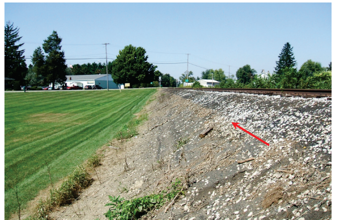
Figure 5. Examples of lines used as high-water marks at selected locations in the flooded area. A , Seed line on buildings or trees. B , Mud lines on buildings. C , Debris lines on fence or ground.
