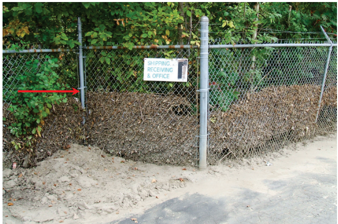
Figure 5. Examples of lines used as high-water marks at selected locations in the flooded area. A , Seed line on buildings or trees. B , Mud lines on buildings. C , Debris lines on fence or ground.
