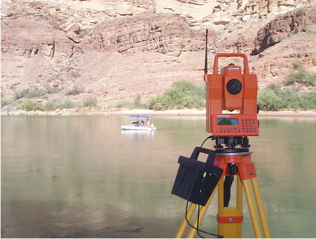
Figure 4. Photograph of the Spectra Precision Geodimeter ATS-PT robotically tracking the survey raft.
