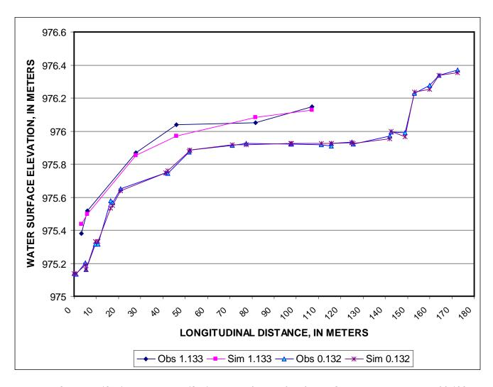
Figure 37. Observed (Obs) and simulated (Sim) water surface profiles for the Gage site at discharges of 0.132 and 1.133 m<sup>3</sup>/s (4.65 and 40 ft<sup>3</sup>/s).
