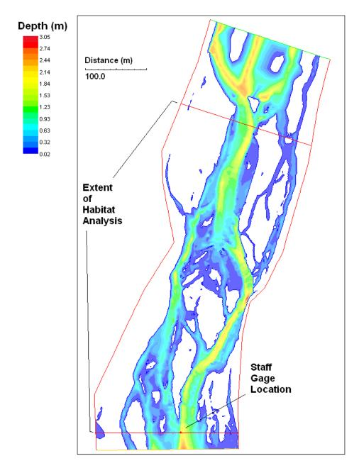
Figure 42. Depth distribution for Braided site for a simulated discharge of 3,800 ft<sup>3</sup>/s (107.8 m<sup>3</sup>/s)
