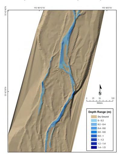
Figure 5. Depth TIN for the lower (Braided) site at Cherry Creek for a discharge of 10 ft<sup>3</sup>/sec.
