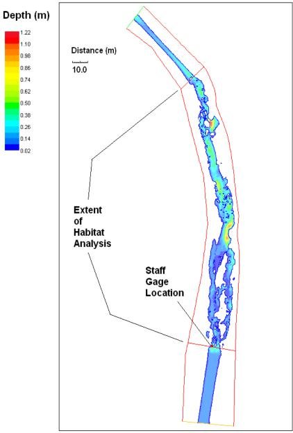
Figure 40. Depth distribution at Gage site for the 0.132 m³/s (4.67 ft³/s) discharge.
