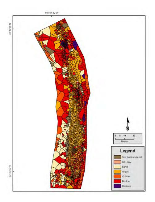
Figure 8. Substrate polygon map for the upper (Gage) study site resulting from proximity analysis using the Thiessen polygon algorithm.
