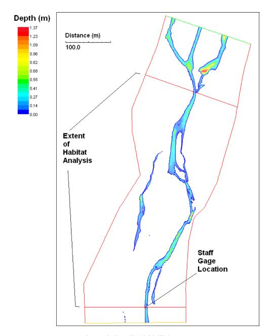
Figure 41. Depth distribution at Braided site for the 0.137 m<sup>3</sup>/s (4.84 ft<sup>3</sup>/s) discharge.
