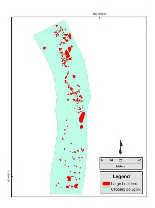
Figure 10. Shapefile for the upper (Gage) site showing polygons for individually-surveyed large boulders.
