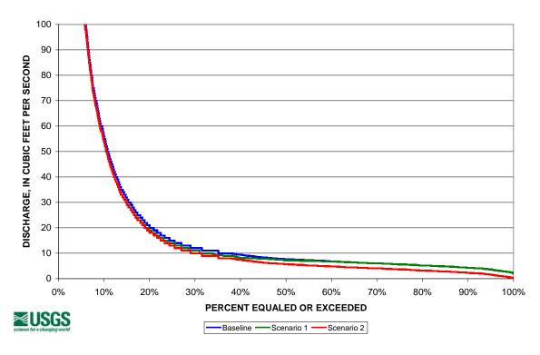
Figure 52. Flow duration curve for the Gage site under baseline conditions and scenarios 1 and 2, assuming a hypothetical diversion of 2 ft<sup>3</sup>/s.
