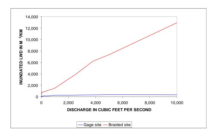
Figure 78. Inundation of LWD as a function of discharge at the two study sites.
