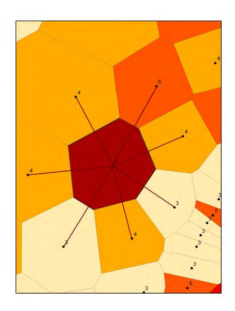
Figure 7. Radiating lines from a point to its nearest neighbors, perpendicularly bisected to form the boundaries of the Thiessen polygon shown as dark red. Here the numbers indicate substrate codes observed at the respective points.
