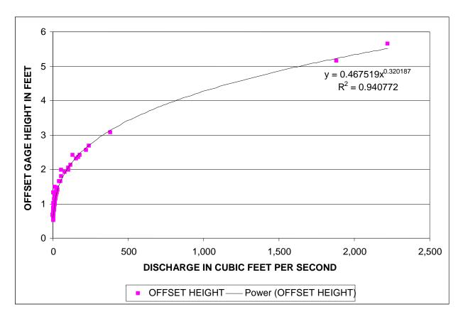
Figure 3. Observed gage height offset by -1.15 ft and power function fit.
