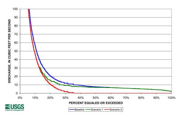
Figure 54. Flow duration curve for the Gage site under baseline conditions and scenarios 1 and 2, assuming a hypothetical diversion of 10 ft<sup>3</sup>/s.
