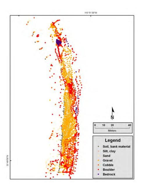
Figure 6. Map of the upper (Gage) study site showing topographic survey points and substrate codes.
