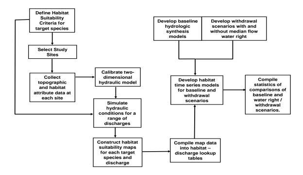
Figure 2. Analytical process flow chart.
