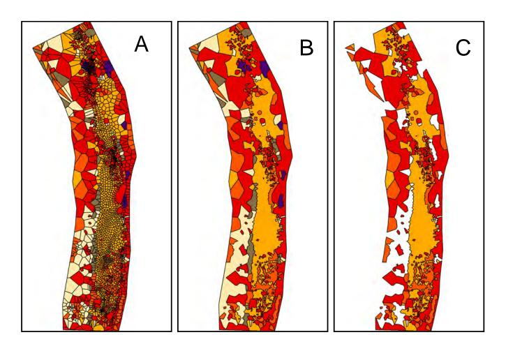
Figure 12. Comparison of original Thiessen substrate polygons with boulder inserts (*A*), merged substrate polygons (*B*), and resultant substrate polygons suitable for speckled dace (*C*).
