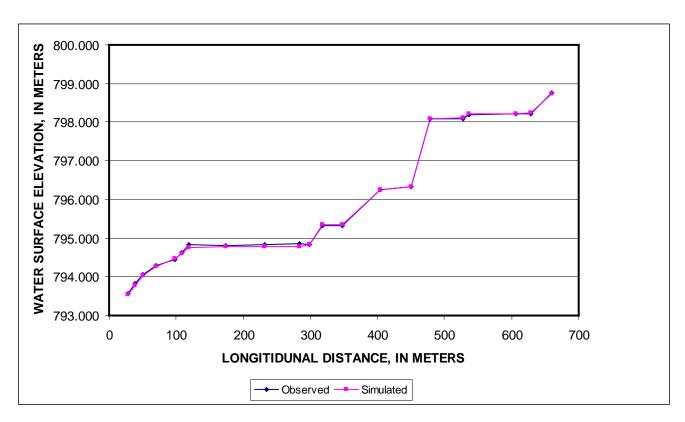
Figure 38. Observed and simulated water surface profiles for the Braided site at 0.137 m<sup>3</sup>/s (4.84 ft<sup>3</sup>/s).
