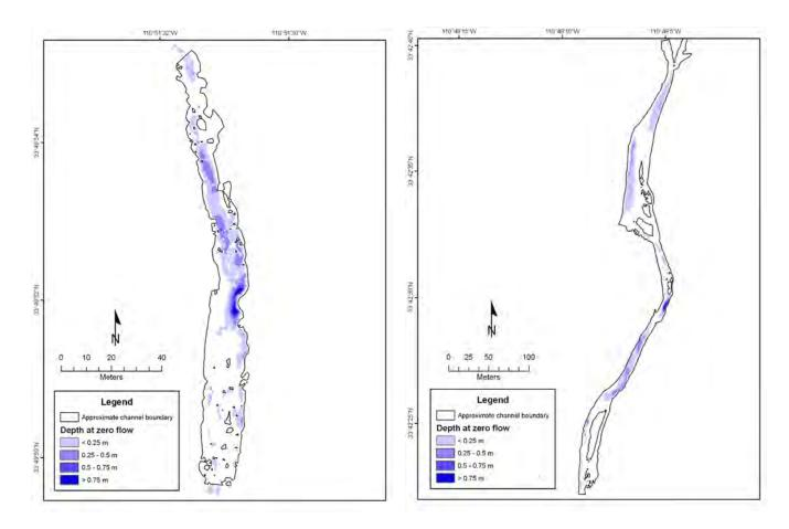
Figure 77. Depths of pools at zero discharge in the Gage site (left) and Braided site (right).
