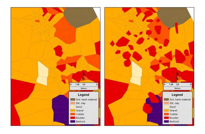
Figure 11. Close-up comparison of the base substrate map from Thiessen polygons (left) and final substrate map with replacements for large boulders (right) for the upper (Gage) site.
