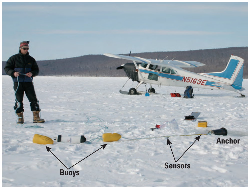
Figure 5. Buoys, sensors, and anchor used to measure temperature in Wonder Lake, Chilchukabena Lake and Lake Minchumina, Alaska. Photograph taken by Daniel A. Long, 2007.
