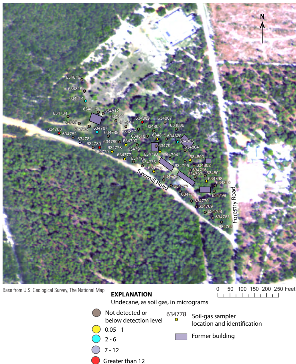
Figure 7. Detections of undecane mass in soil-gas samplers, Old Metal Workshop Hog Farm Area, Fort Gordon, Georgia, 2009–2010.
