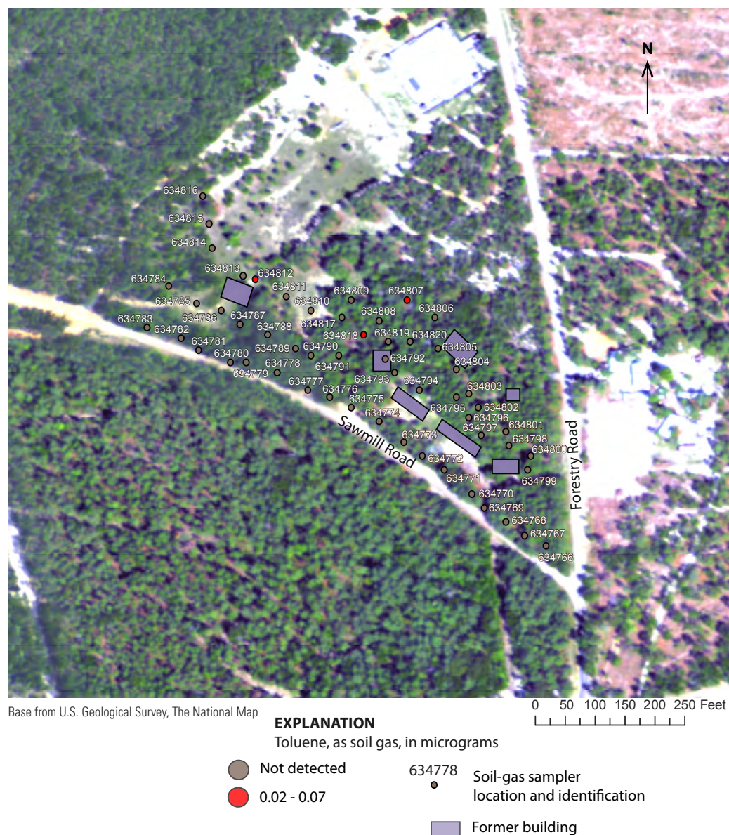
Figure 8. Detections of toluene mass in soil-gas samplers, Old Metal Workshop Hog Farm Area, Fort Gordon, Georgia, 2009–2010.
