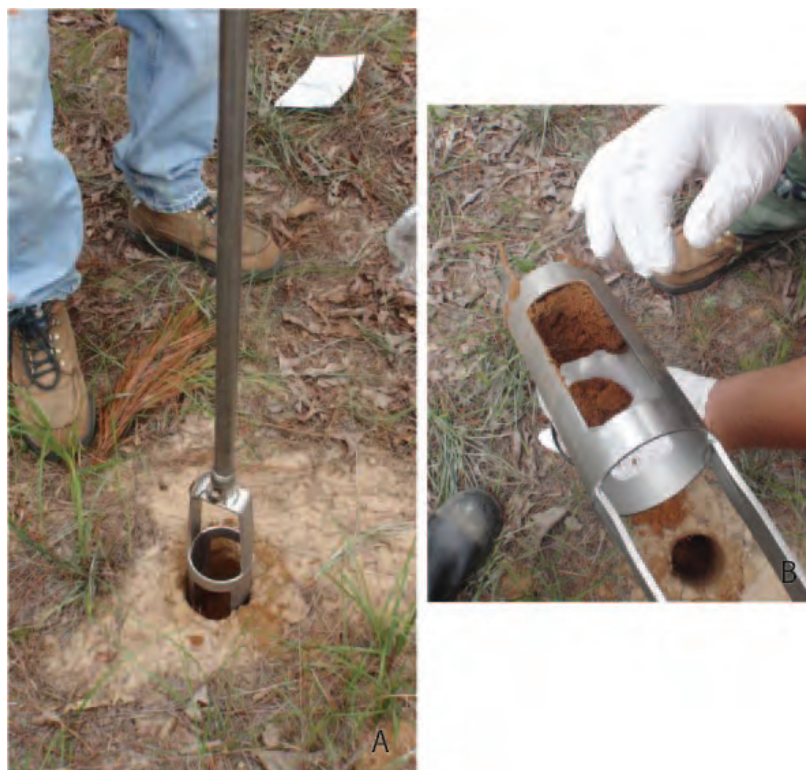
Figure 5. Soil sample (A) extracted with stainless-steel auger and (B) transferred to sample container.
