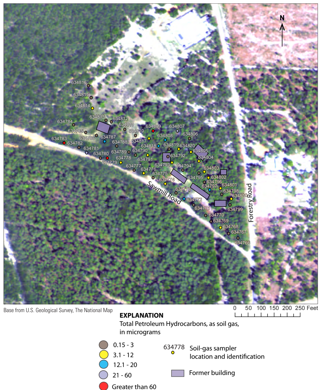
Figure 6. Detections of total petroleum hydrocarbon mass in soil-gas samplers, Old Metal Workshop Hog Farm Area, Fort Gordon, Georgia, 2009–2010.
