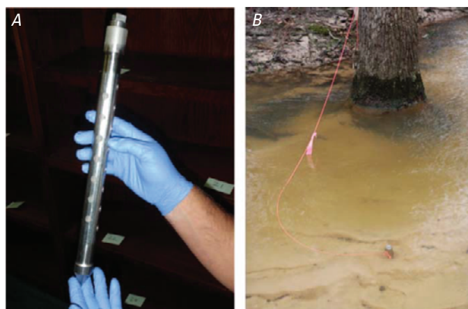
Figure 5. An example of a hyporheic-zone sampler showing (A) the vented stainless-steel drive point and cap used to house the passive soil-gas sampler and (B) a deployed sampler inserted into the creek-bed sediments (the top of the deployed sampler is attached to the submerged end of the pink string in the photograph).
