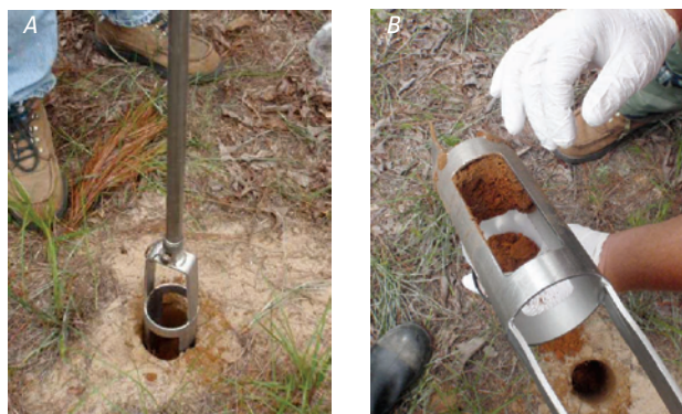
Figure 7. Soil sample (A) collected in the interval from land surface to a depth of 6 inches with a stainless-steel hand auger and (B) transferred from the auger to a plastic container for shipment to the laboratory.
