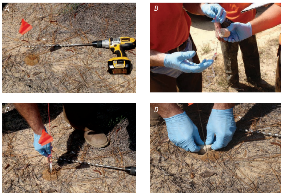
Figure 6. Installation of a passive soil-gas sampler in the landfill soil consisted of (A) drilling a borehole in the soil with a stainless-steel drill bit attached to a cordless drill, (B) attaching one end of a string to the soil-gas sampler and the other end to a cork plug, (C) inserting the soil-gas sampler into the borehole, and (D) sealing the borehole with the cork plug to keep out surface material and water.
