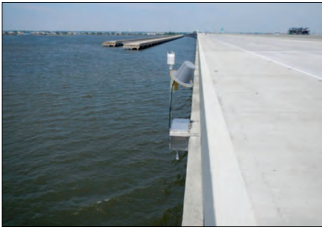
Figure 4. A USGS rapid-deployment gage collecting real-time water-level and meteorological data at Lake Pontchartrain, Louisiana. Photo by Christopher A. Smith, USGS.
