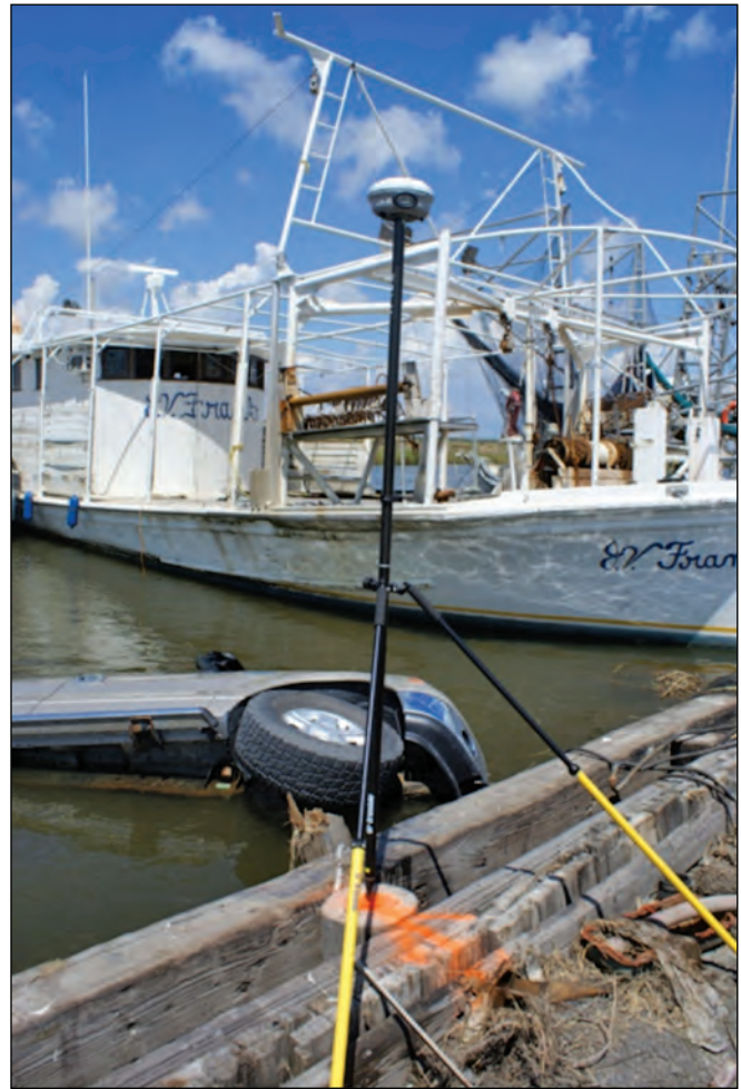
Figure 5. A global positioning system used to survey storm-tide elevation after Hurricane Isaac. Photo by William C. Vervaeke, USGS.
