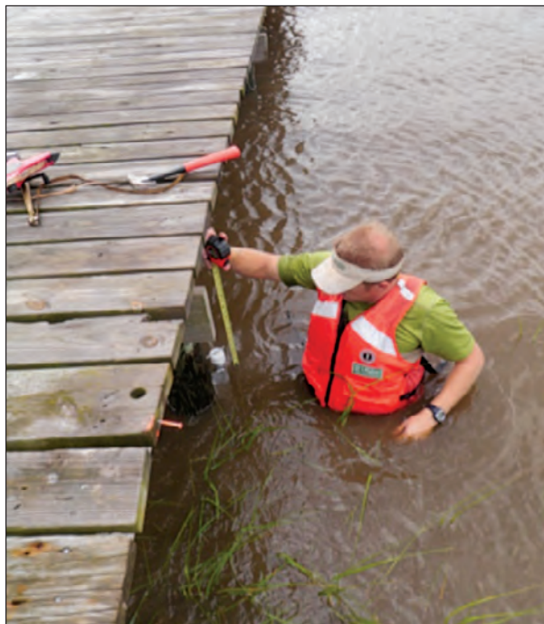
Figure 2. A USGS scientist obtaining water-surface elevation data relative to a known reference elevation and deploying a storm-tide sensor at SSS-MS-JAC-039WV on the west side of Pascagoula Bay in Mississippi, August 28, 2012. Photo by Robert Brendlinger III, USGS.
