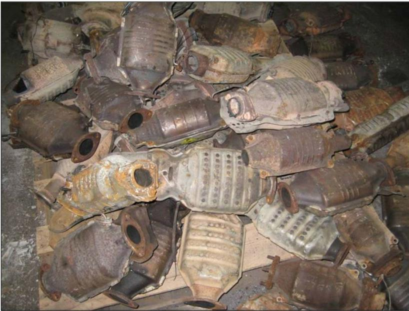
**Figure 1.** Stockpiled catalytic converters (CATCONs) that have been removed from vehicles before the CATCONs were dismantled and recycled for platinum-group metals. Photograph courtesy of Ashok Kumar, Director, A-1 Specialized Services & Supplies, Inc. Used with permission.
