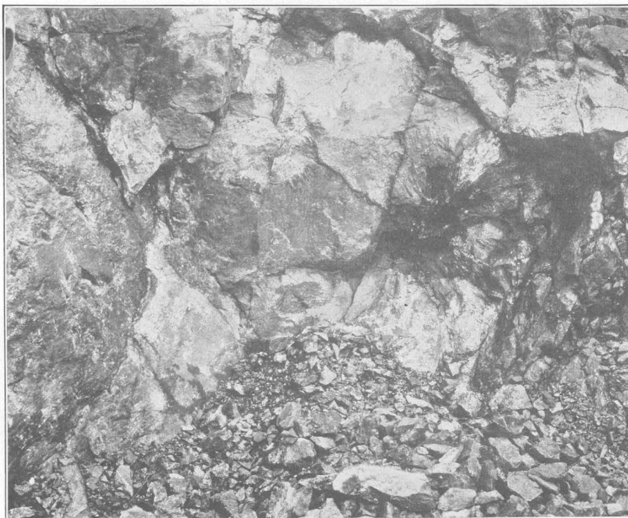
B. MASS OF CHALCOPYRITE ORE INCLOSED IN CONTACT ROCK. Dark patch on right is massive chalcopyrite. View taken just above mouth of tunnel No. 2, Jumbo claim No. 4.
