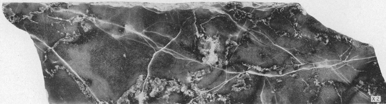
A. METALINE LIMESTONE, PEND OREILLE MINE. Polished fragment of split drill core, 140 feet below Le Hetter slate.
