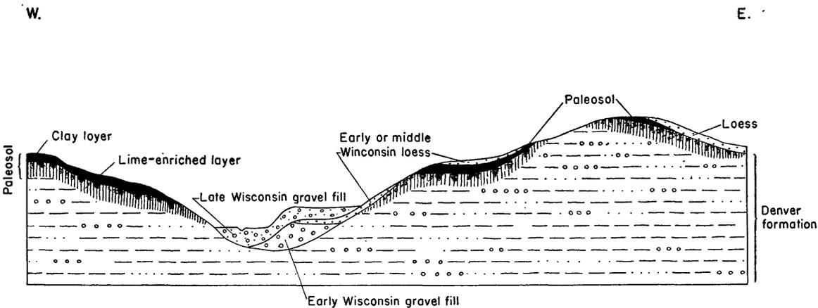
FIGURE 13.—Diagrammatic cross section illustrating topographic and stratigraphic relations of the paleosol in the Denver Basin. Paleosol has developed on the Denver formation and on old surficial deposits (not shown) that lie on the Denver. The paleosol is older than the loess and must be older than the early Wisconsin gravel fill, which was the source of the loess.
