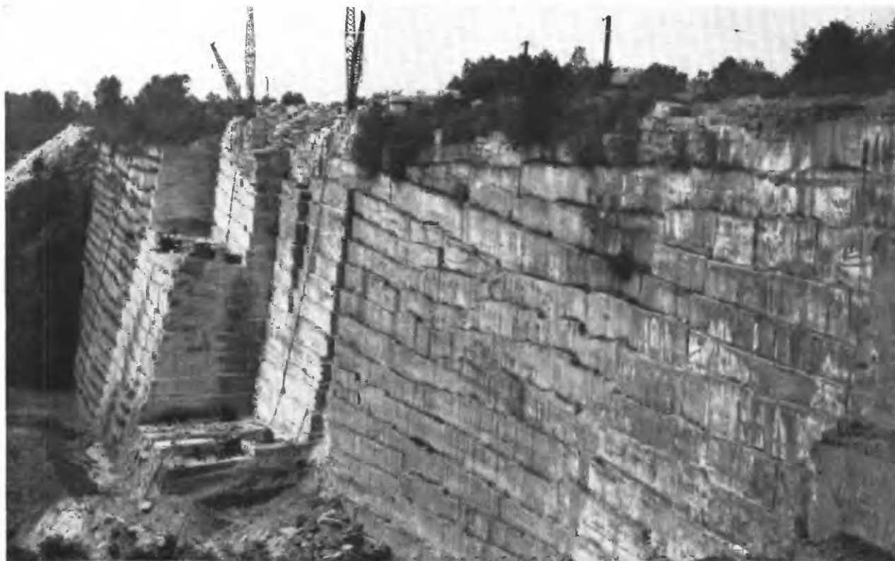
FIGURE 14.—The north wall of the Buckeye quarry, South Amherst, Lorain County, Ohio. About 150 feet of Berea sandstone is exposed in this photograph. Less than 300 feet back from the quarried face, core drilling recorded only red Bedford shale.
