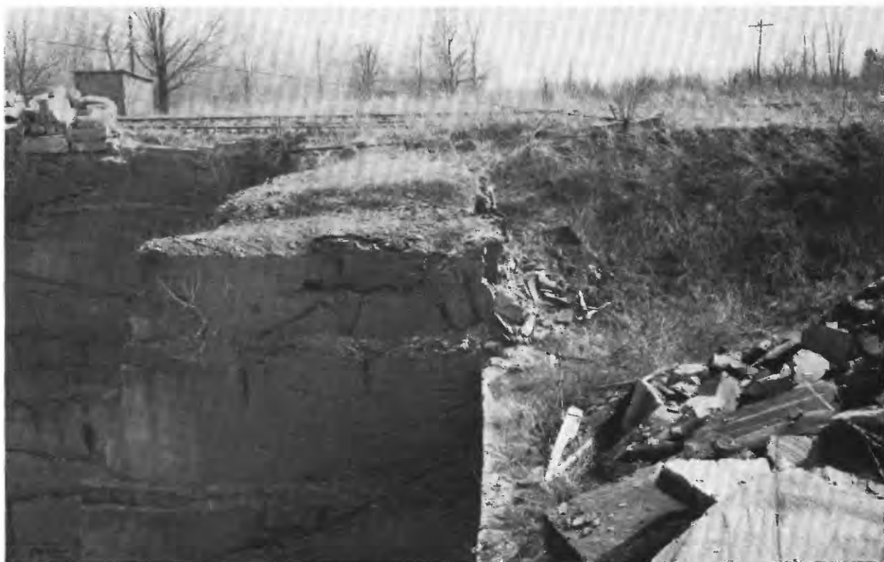
FIGURE 16.—Southeast corner of the Nicholl quarry at Kipton, Camden Township, Lorain County, Ohio. View illustrates the steep wall of one of the thicker sandstones of the Berea. The man is seated on Berea sandstone which core-drill records show has a minimum thickness of 100 feet. The red Bedford shale is exposed in the small excavation to his left. A drill-hole core, 20 feet to the man's left, showed only red shale and no sandstone. Figure 39 shows the relative location of the Nicholl and Buckeye quarries.
