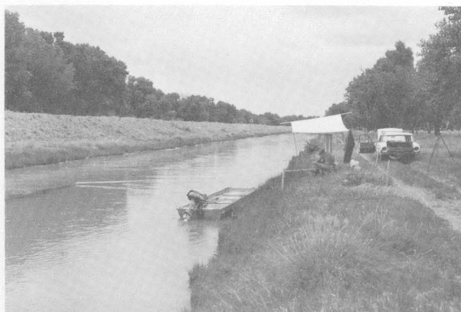
FIGURE 1.—View of Atrisco Feeder Canal, near Bernalillo, N. Mex., showing channel conditions at a discharge of 269 cubic feet per second, June 21, 1966. Centerline injection of dye is shown on the left (at end of white pipe).
