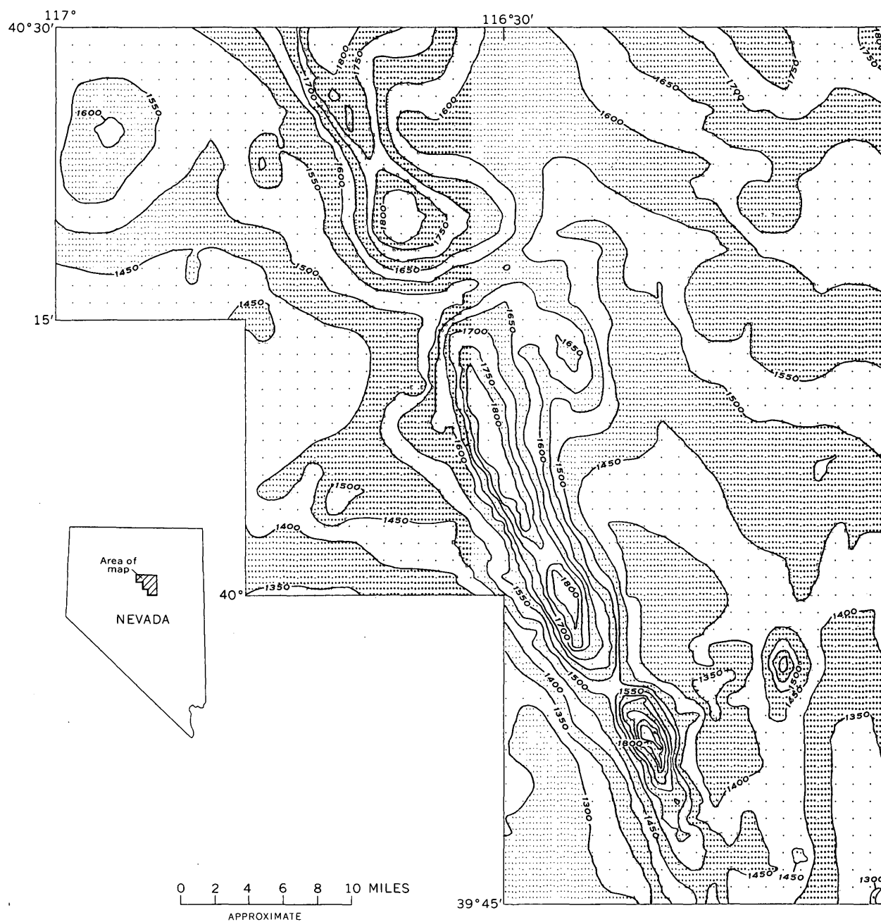
FIGURE 4.—Aeromagnetic map of part of central Nevada digitized on a 1-mile grid and plotted with high-speed printer. Contour interval is 50 gammas. Illustration is a reduced composite of computer printout sheets to which contours have been added.
