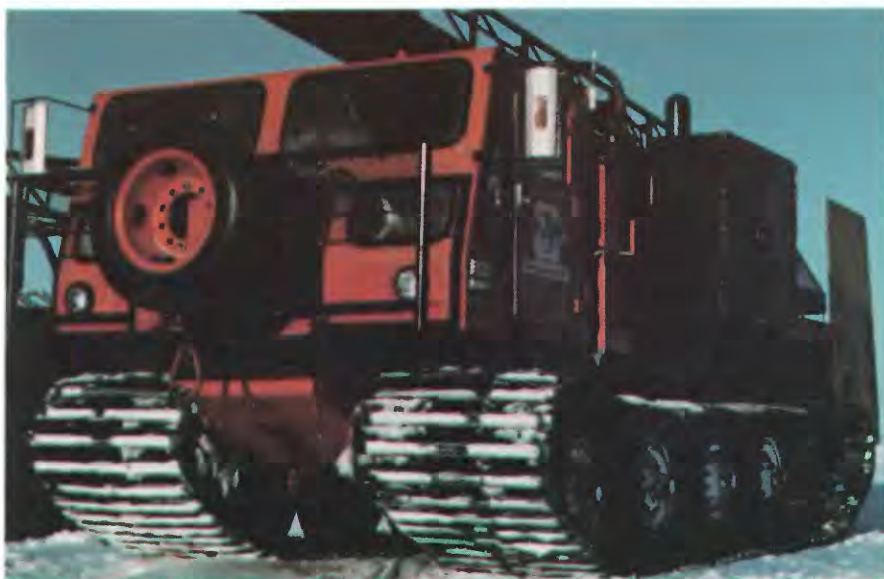
FIGURE 2.11.—Seismic drill rig mounted on Nodwell vehicle, spring 1975. Photograph by U.S. Navy.
