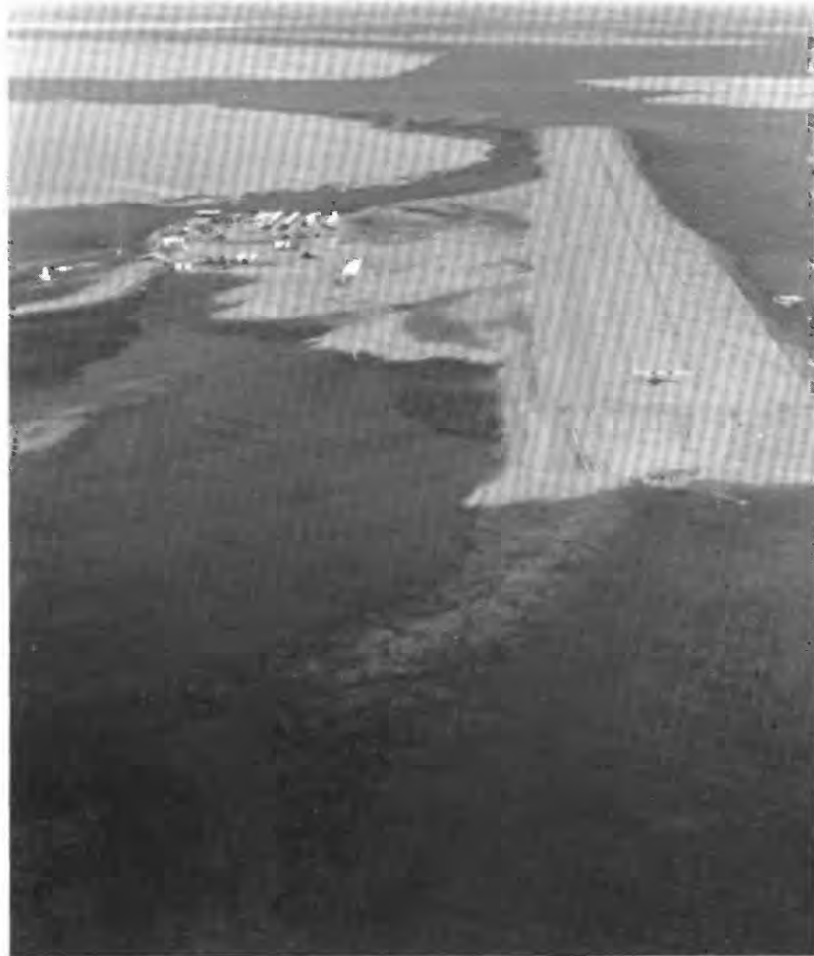
FIGURE 38.6.—The all-season airstrip at Inigok, showing insulated runway, taxiway, parking apron, and road to drill site. Darker area along road was result of tundra fire in 1977. View looking northeast taken in July 1978.
