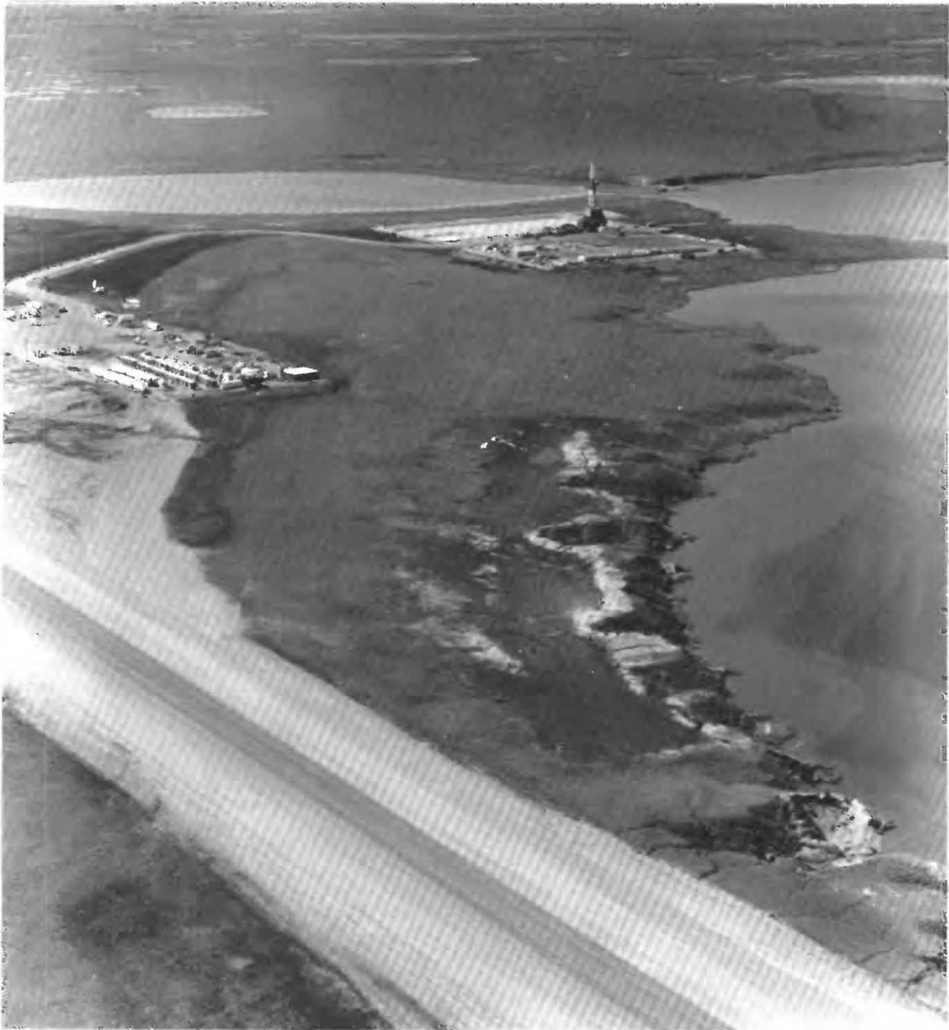
FIGURE 38.4.—Inigok well site, road, and airstrip. Area on runway centerline darker because sprinkled with water. Large lake on right used as airstrip in winter. View looking westward in July 1978.
