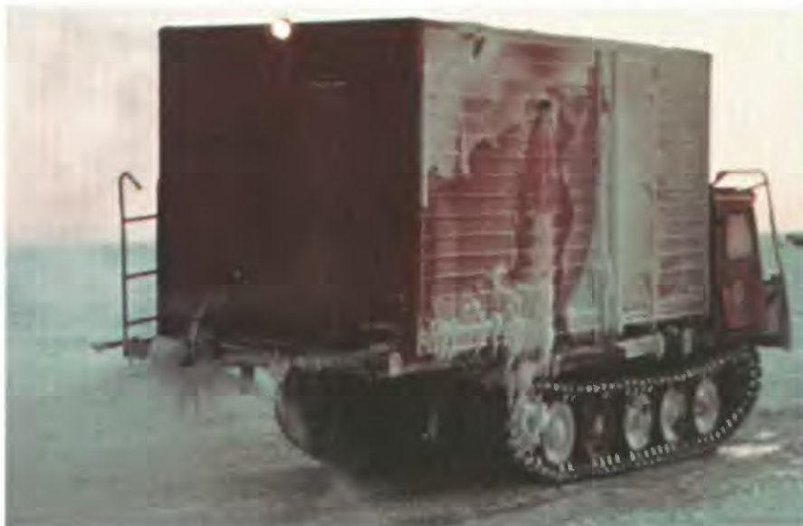
FIGURE 2.15.—Spraying water to build ice road at South Simpson, January 1977.
