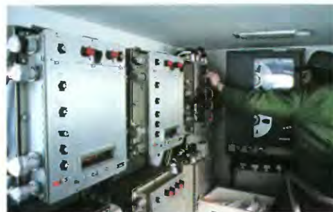
Inside the seismic recording trailers, where the sonic waves are recorded and plotted.
