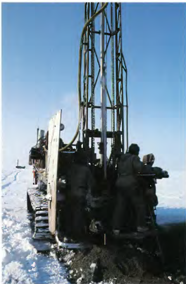
Drill holes for shot emplacement to create sonic waves.
