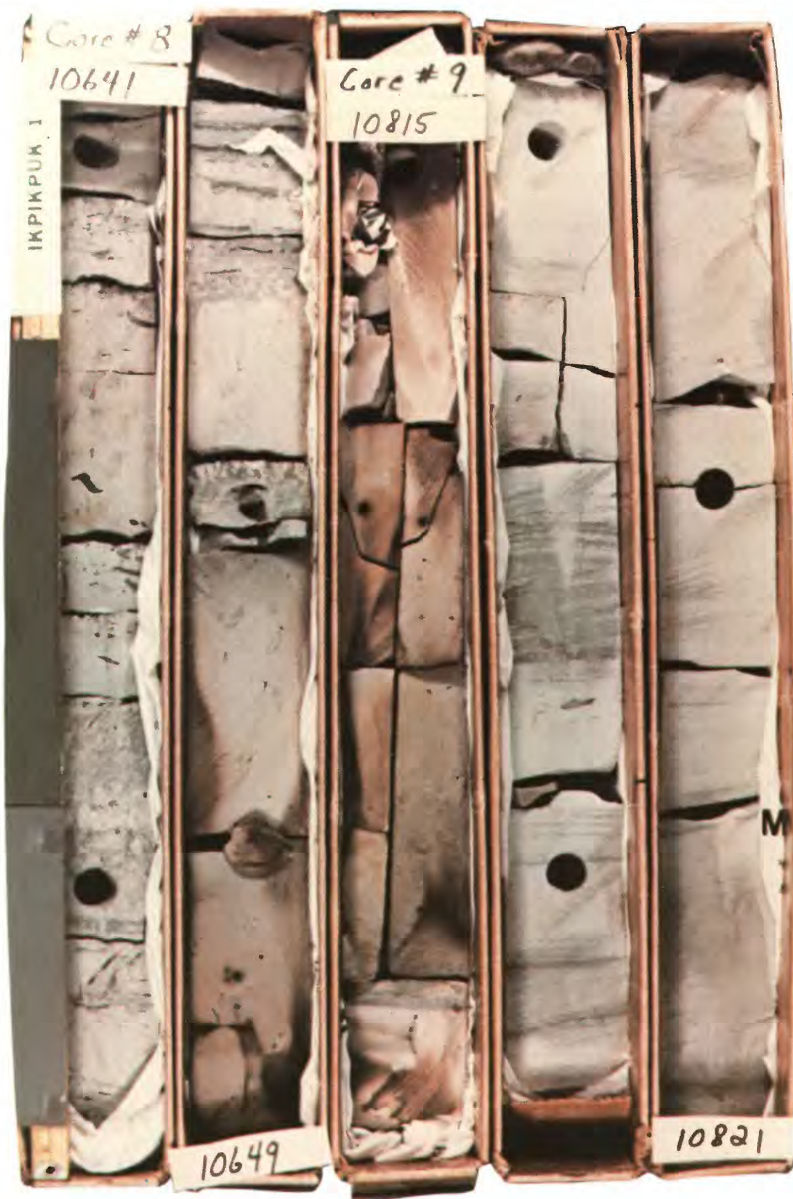
Typical cores of potential reservoir rocks from the Ikpiuk No. 1 well, at depths of 3243 to 3246 m (10,641-10,649 ft) and 3296 to 3299 m (10,815-10,821 ft) in the Ivishak Formation. Holes are where plugs were drilled to determine porosity and permeability. The Ivishak Formation is the main producing horizon at the Prudhoe Bay oil field.
