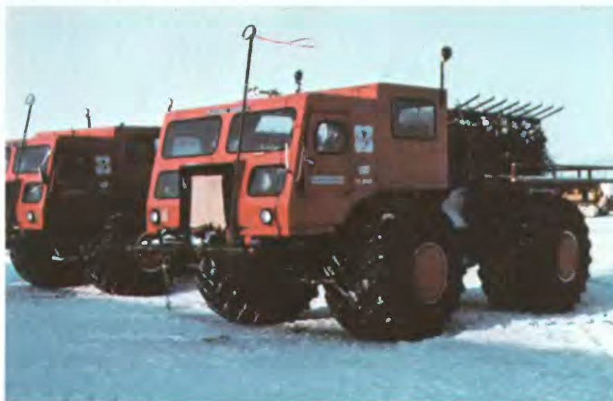
FIGURE 2.10.—All-terrain vehicles used by seismic trains in the NPRA, spring 1975. Note racks on rear bed to hold geophones. Photograph by U.S. Navy.
