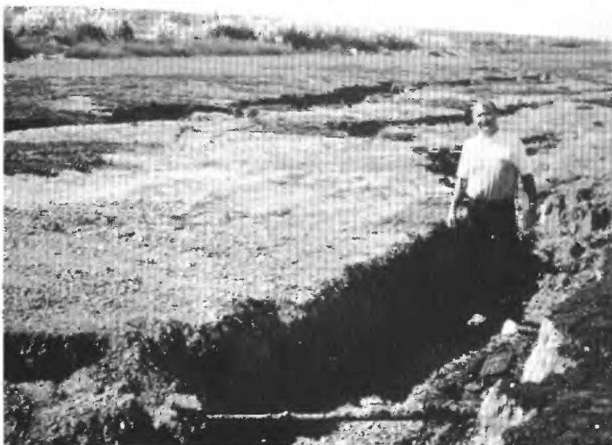
Figure 24.—Fissures, sand boils, and grabens associated with lateral spreading near north-west end of main runway at Oakland International Airport. Photograph courtesy of B.A. Vallergera.
