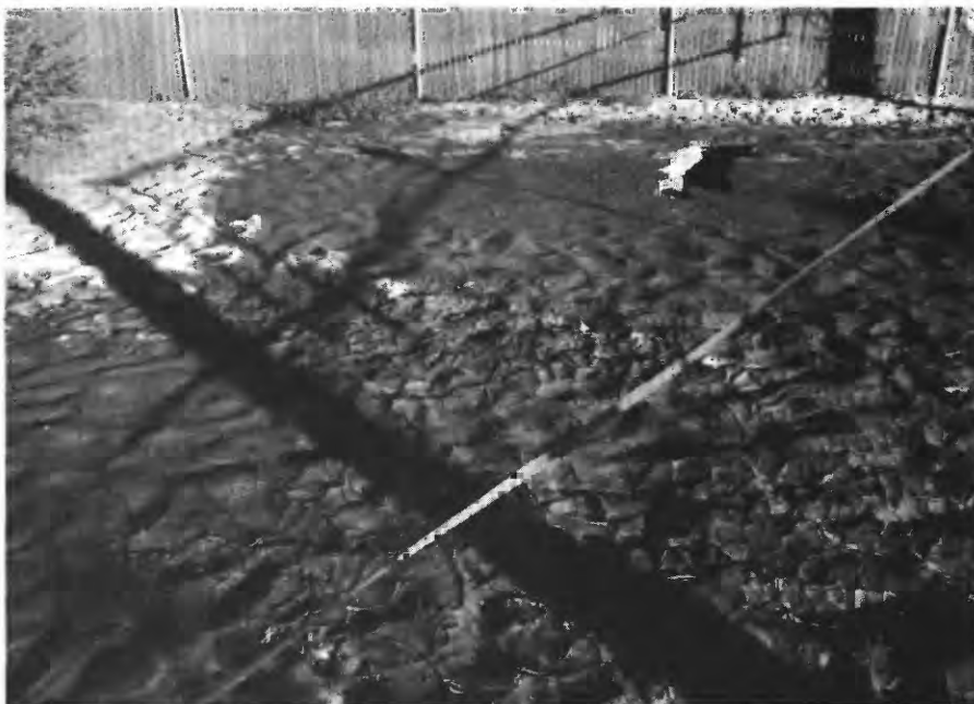
Figure 15.—Sand-boil ejecta in volleyball court of Moss Landing Marine Laboratory (fig. 11).
