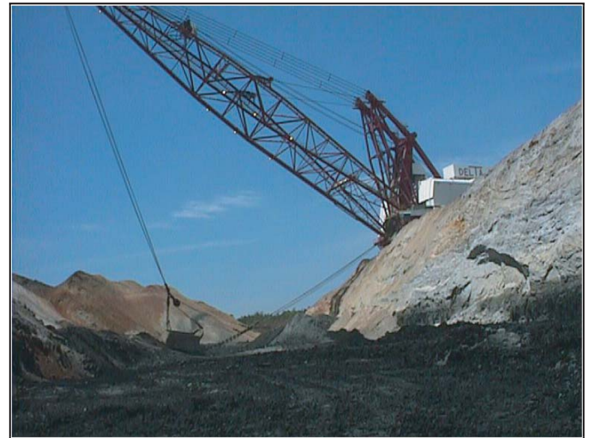
A dragline being used to remove overburden in Gulf Coast mines.
