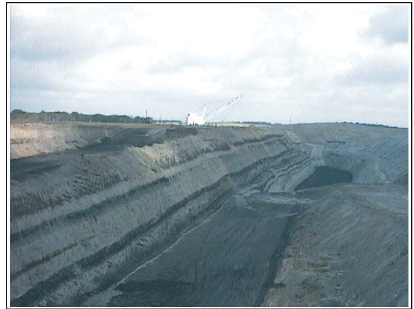
View of a mine pit in the Gulf Coast coal region. The top of the coal bed being mined is exposed at the far end of the pit.
