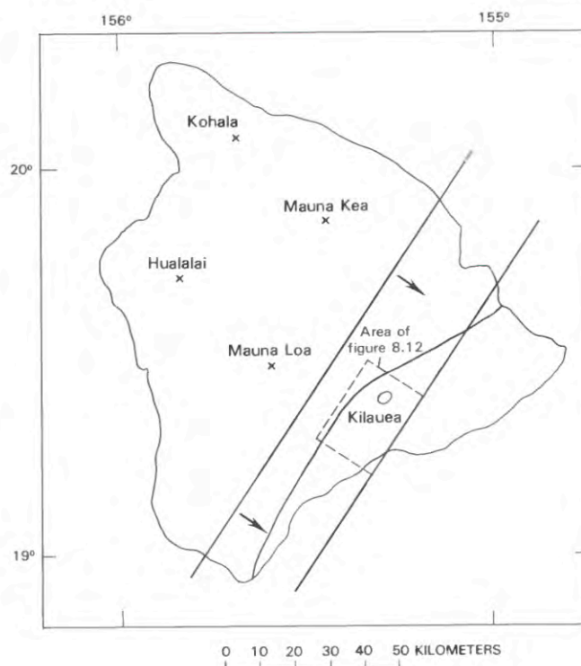
FIGURE 8.11.—Location of SIR-B radar images (area between parallel lines) that were acquired over southeast Hawaii in October 1984. Radar look-direction (arrowed) was toward southeast, and Shuttle flew from southwest to northeast on both data takes.
