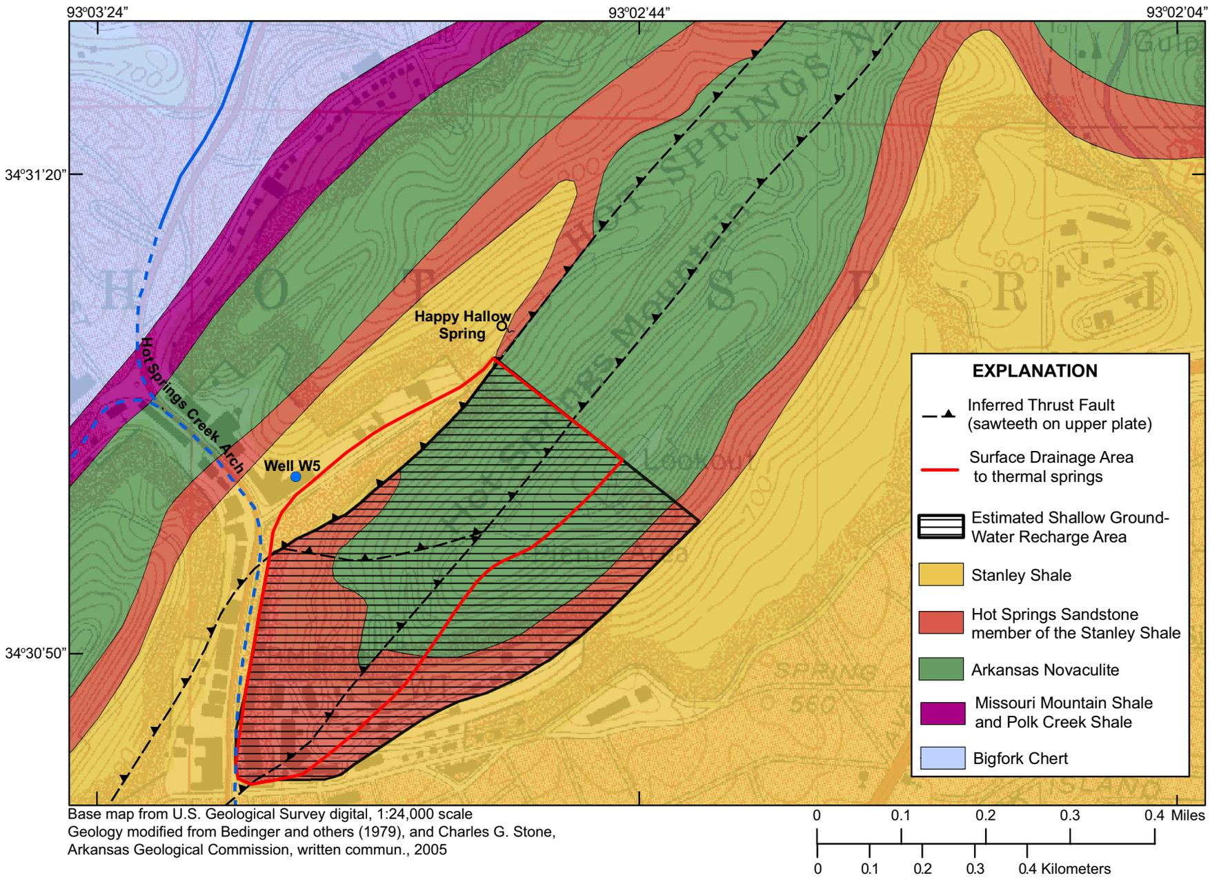
**Figure 15.** Estimated recharge area for shallow ground-water contribution to the thermal springs.
