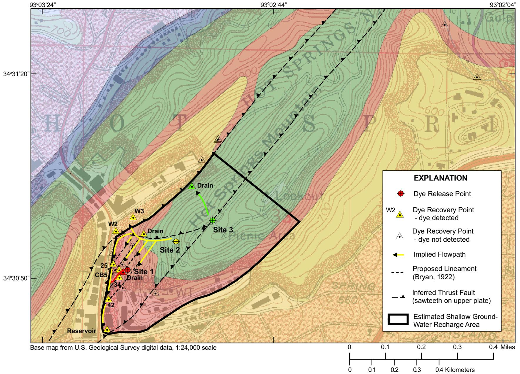
**Figure 16.** Dye release and detection points and implied flow paths of the dyes.
