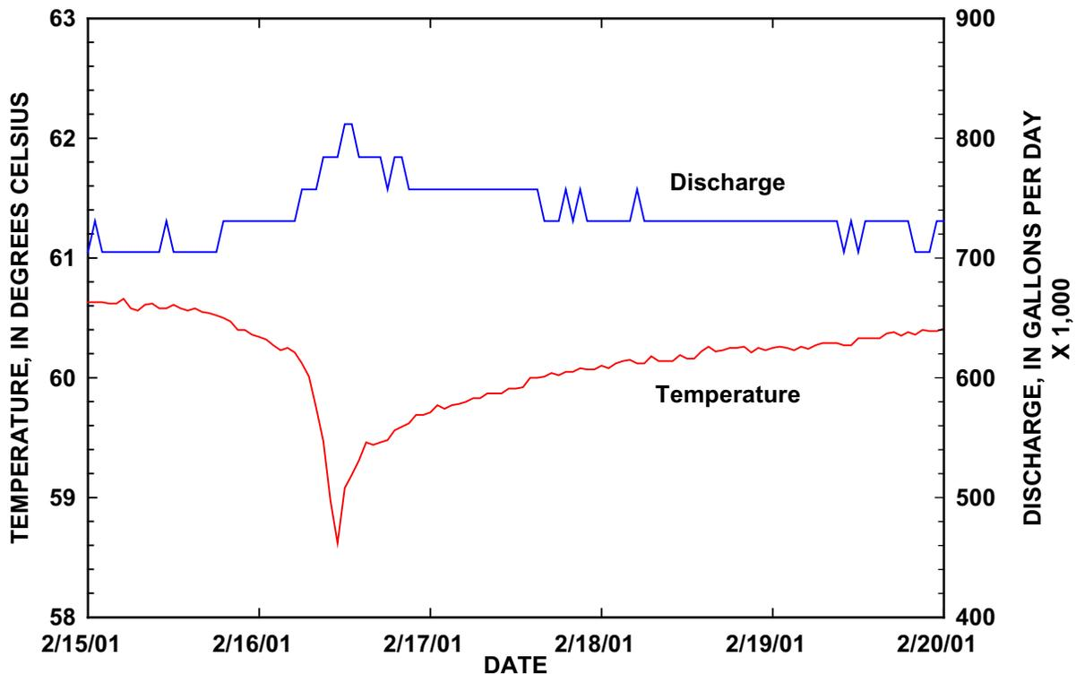
**Figure 8.** Thermal springs collection system hourly temperature and discharge response to 3.5 inches of rainfall on February 15-16, 2001.
