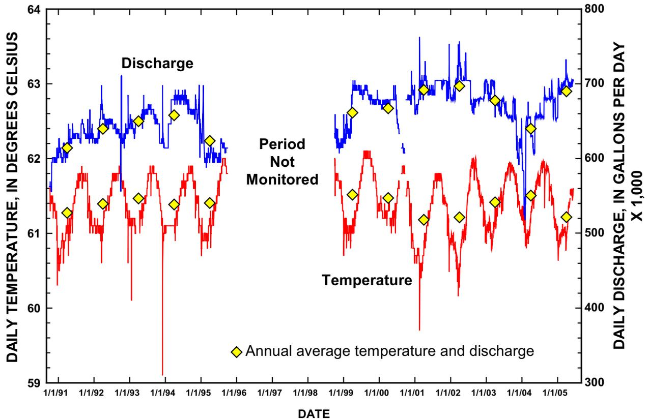
**Figure 7.** Daily and annual average discharge and temperature of the thermal springs at the inflow of the collection system reservoir.
