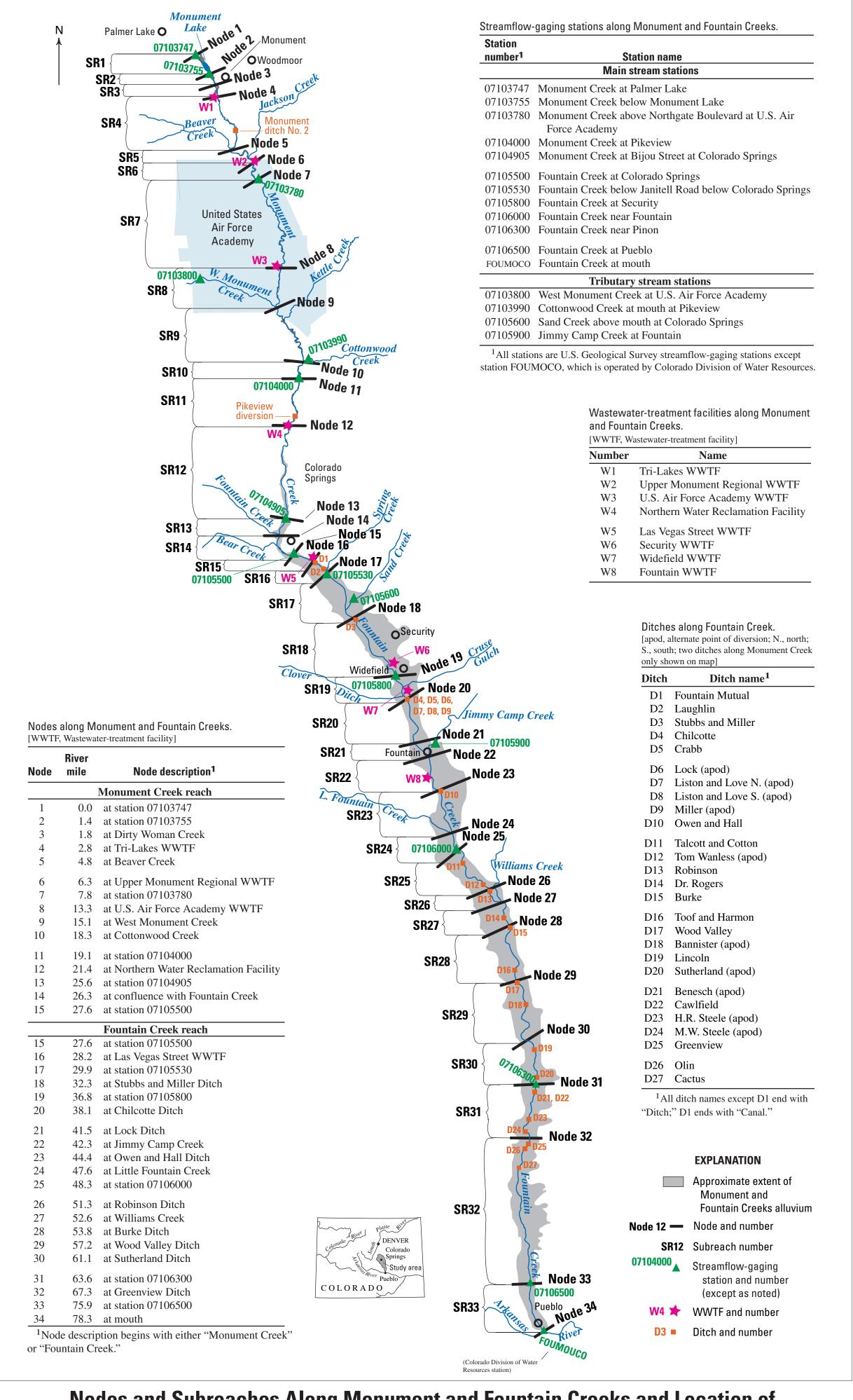
Nodes and Subreaches Along Monument and Fountain Creeks and Location of Streamflow-Gaging Stations, Wastewater-Treatment Facilities, and Diversions Used in New Transit-Loss Accounting Program
