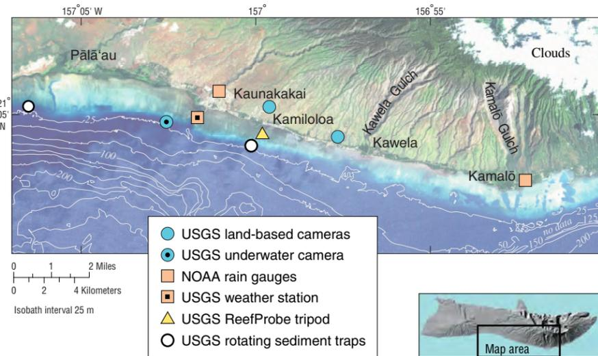
**Figure 1.** Aerial photograph of central south Moloka‘i and the adjacent reef, showing the locations of the U.S. Geological Survey instruments and cameras and the National Oceanic and Atmospheric Administration rain gauges that recorded information during the November 27, 2001, Kona storm. Much of the sediment delivered to the coast in the storm was discharged from Kawela and Kamalō Gulches and other drainages.
