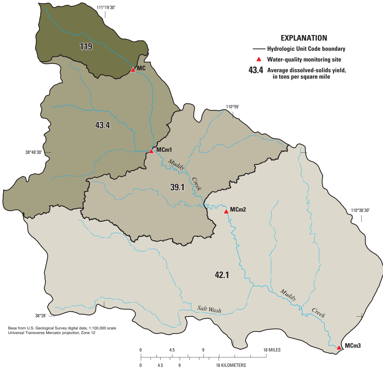
Figure 16. Dissolved-solids yields, in tons per square mile, from selected subbasins of the Muddy Creek Basin, Utah, 2006.
