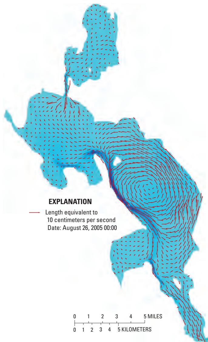
Figure 9. Simulated depth-averaged currents under reversed (southwest) wind conditions, Upper Klamath Lake, Oregon.
