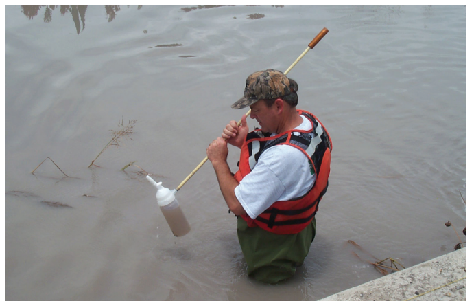
Figure 5. Suspended-sediment sample collection at station West Oso Creek at Merrett Road near Corpus Christi, Texas (08211517), June 2, 2006.
