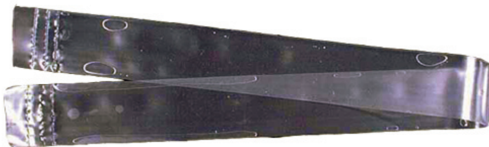
Figure 6. Photograph of lipid-filled polyethylene membrane tube from a semipermeable membrane device (SPMD).
