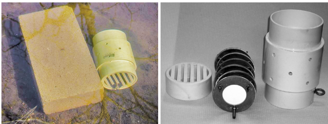
Figure 4. Photographs of passive-sampler canister in stream and with polar organic integrative sampler (POCIS) disks removed.
