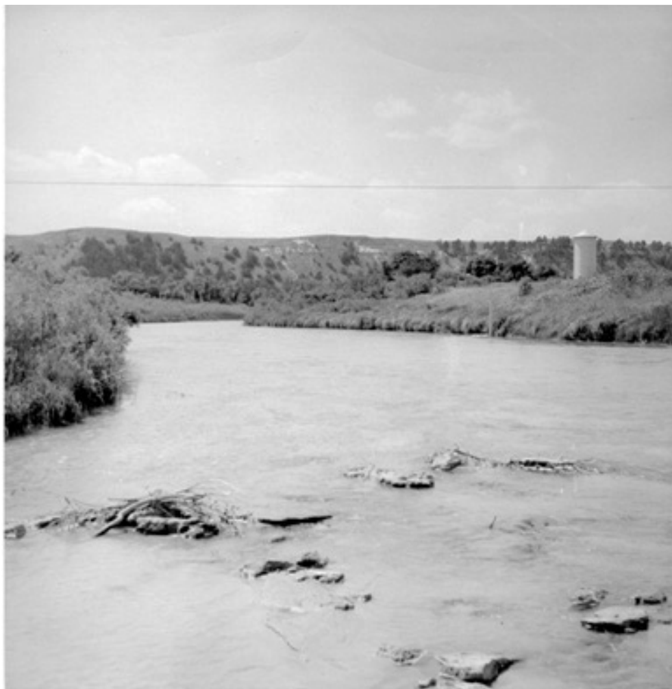
Figure 1-2. Photograph of the Niobrara River near Cody streamflow-gaging station reach. Photo was taken looking upstream. The gage house can be seen on the left river bank (right side of photo). The cableway can be seen one-third distance down from the top of the photo. Most measurements were made by wading underneath the cableway. High-flow measurements were made using the cable car. (USGS file photograph)
