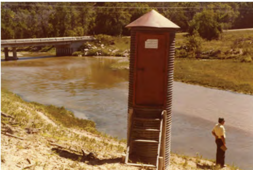
Figure 1-1. Photograph of the Niobrara River near Gordon streamflow-gaging station reach. Photograph was taken looking downstream. The gage house is in the foreground. Many of the measurements were made near the upstream face of the bridge. (USGS file photograph)
