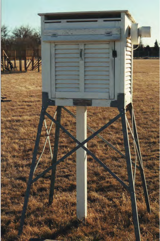
Figure 5. Temperature and humidity sensing system of the National Weather Service.
