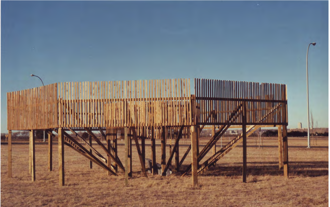
Figure 1. Double fence intercomparison reference having a Tretyakov gage.
