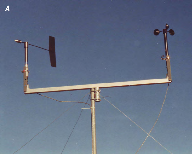
Figure 6. Wind speed and wind direction sensors at 3.0-meter height (A) and wind speed sensor at 1.4-meter height (B).
