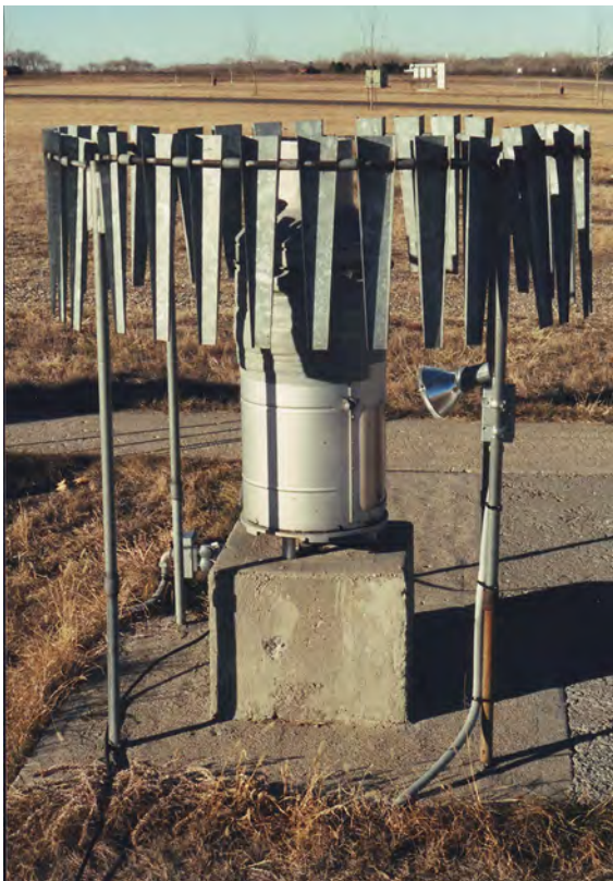
Figure 3. National (National Weather Service) gage equipped with the national standard windshield.
