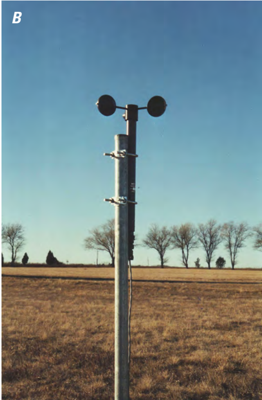
Figure 6. Wind speed and wind direction sensors at 3.0-meter height (A) and wind speed sensor at 1.4-meter height (B).
