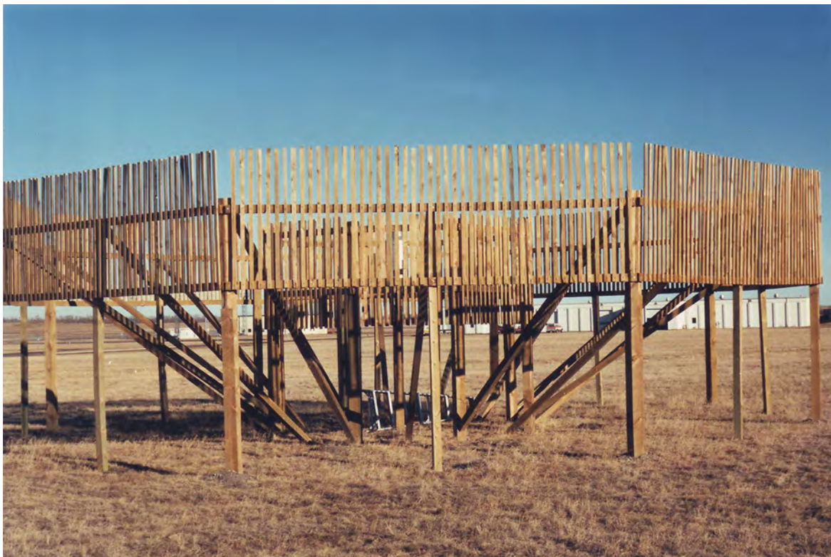
Figure 8. National (National Weather Service) gage with double fence shield.
