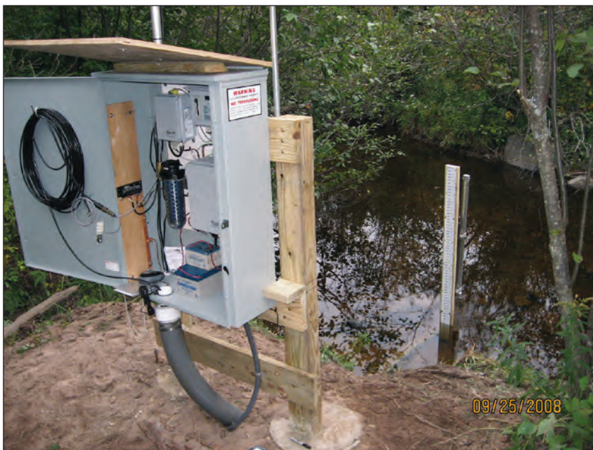
Figure 7. U.S. Geological Survey streamgage at upper Silver River (04043126) during installation. (Photograph by M. A.A. Holmio, U.S. Geological Survey)
