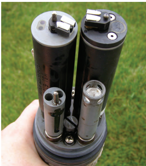
Figure 5. Continuous water-quality monitor with (clockwise from upper left) turbidity, dissolved oxygen, pH, and combined specific conductance and water temperature sensors.
