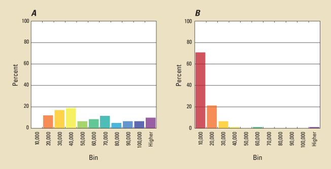
**Figure B3-1.** Distribution of objective functions computed with 100 stochastic parameter realizations (a) before null-space projection and recalibration; (b) after null-space projection. Generally, the post-null-space projected parameter sets can be reconditioned with only a small computational burden.
