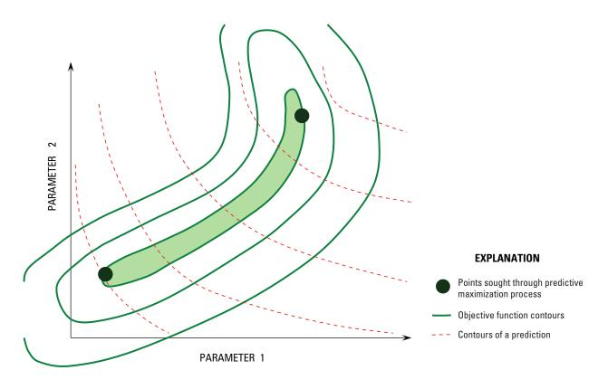
Figure 6. Schematic description of calibration-constrained predictive maximization/minimization.
