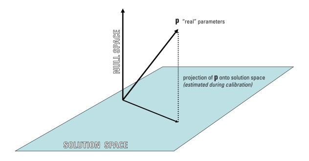
**Figure A4.2.** Relation between real-world and estimated parameters where model calibration is achieved through truncated SVD.
