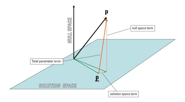
Figure A4.3. Components of postcalibration parameter error.
