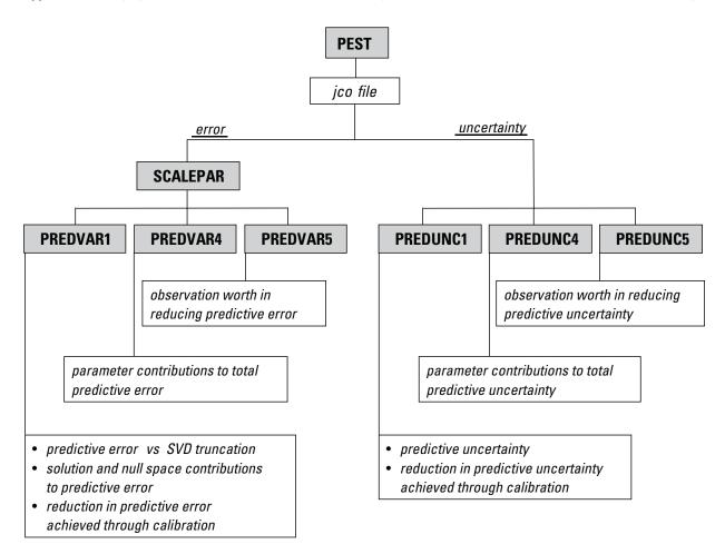
Figure 10. PEST utilities available for calibration-independent error and uncertainty analysis.
