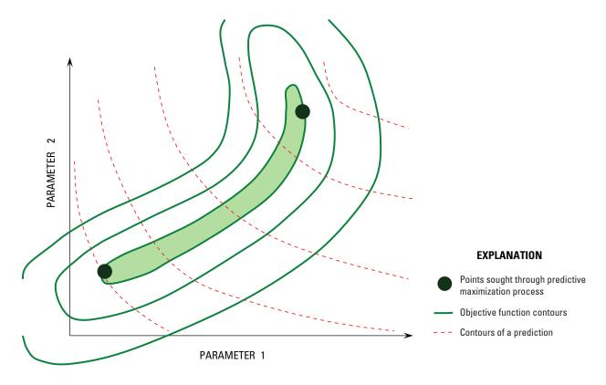
Figure A4.4. Schematic description of calibration-constrained predictive maximization/minimization.
