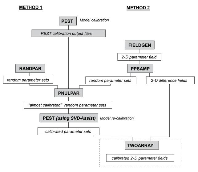
**Figure 13.** Schematic of null-space Monte-Carlo methodologies. Note that in method 2, maximum effectiveness is achieved if the boxed segment through which parameters and two-dimensional difference fields are recombined is included in the model because it is subject to recalibration.
