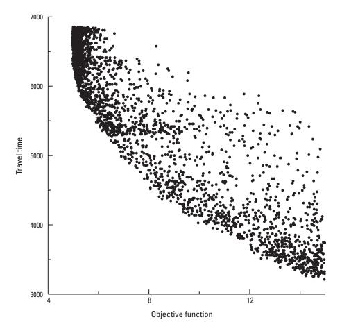
**Figure 8.** A Pareto-front plot of the tradeoff between best fit between simulated and observed targets (objective function, x-axis) and the prediction of a particle travel time. The correct prediction is 3,256 days, which requires an appreciable degradation of the calibrated model in order to be simulated (modified from Moore and others, 2010).
