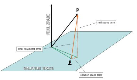
Figure 3. Components of postcalibration parameter error.
