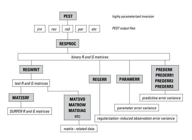
**Figure 9.** Utilities available for postcalibration parameter and predictive error variance analysis. (See appendix 2 for additional description of these utilities.)
