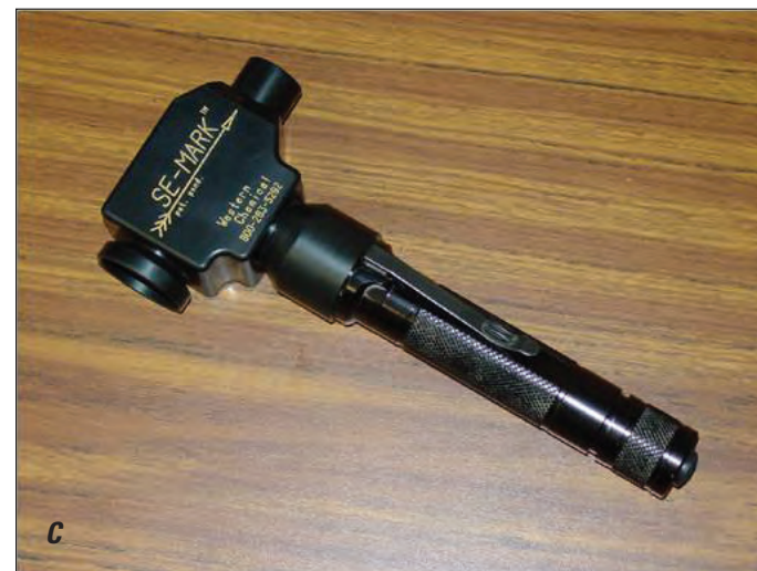
Figure 8. Subyearling Chinook immersed in Calcein solution, recovery after marking, and the Calcein detector. (Photographs taken by Ryan Koch, U.S. Geological Survey, April 22, 2004.)
