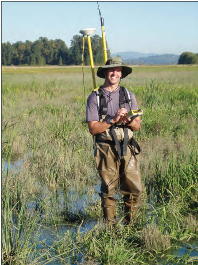
Figure 9. RTK GPS instruments used for surveying the topography and bathymetry of the Restoration site pre- and post-restoration, Columbia River estuary, Oregon. (Photographs taken by John Olson and Craig Haskell, U.S. Geological Survey, October 11, 2006.)
