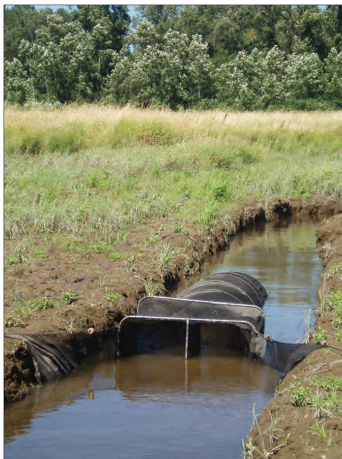
Figure 5. Small fyke net used for sampling intertidal channels post-restoration, Columbia River estuary, Oregon. (Photograph taken by John Olson, U.S. Geological Survey, July 27, 2006.)
