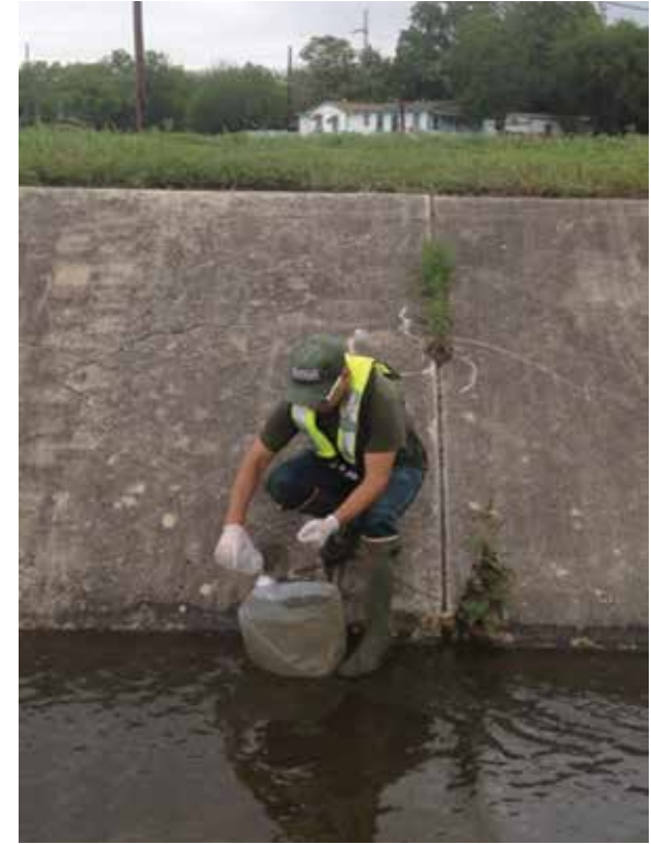
Figure 3. A , streambed-sediment sample collection; B , processing (from Wilson, 2016); and C , collection of water samples for toxicity-testing used at sites in the Westside Creeks (Alazán, Apache, Martínez, and San Pedro Creeks) and San Antonio River, San Antonio, Texas, 2014.
