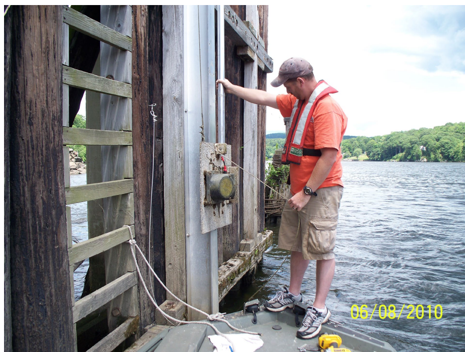
Figure 3. The side of a fuel pier in the Connecticut River with an acoustic Doppler velocity current profiler and the rail system on which it was mounted. Photograph by Joseph Martin, U.S. Geological Survey.
