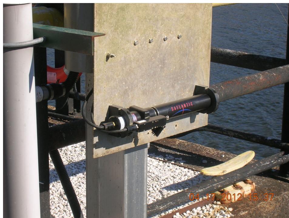
Figure 5. The sensor array to measure nitrate plus nitrite nitrogen mounted to a fuel pier in the center of the Connecticut River at Middle Haddam, Conn. Photograph by Joseph Martin, U.S. Geological Survey.
