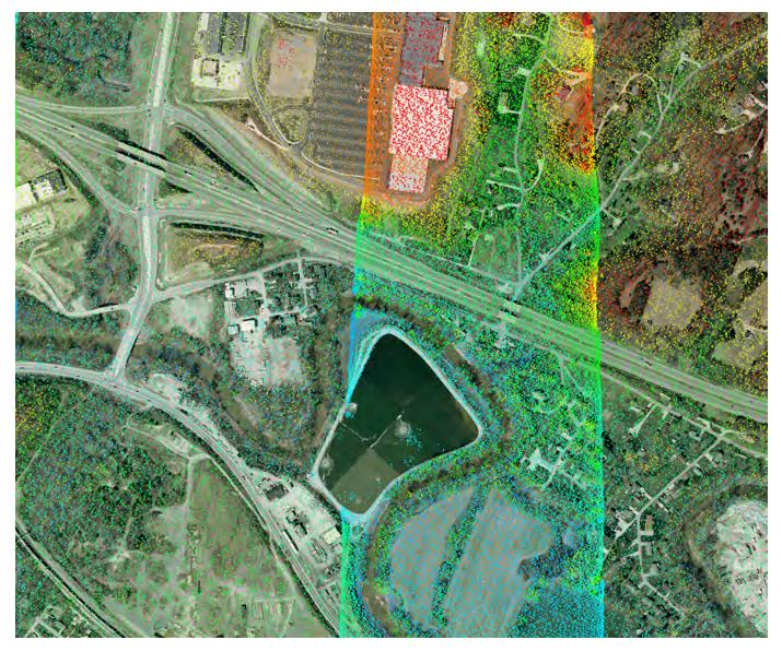
**Figure 7.** Sample area overlaid with light detection and ranging points. This demonstrates the point coverage colored by elevation from blue (low) to red (high). The point density has been dramatically reduced in this image to allow the base image to remain visible. Image courtesy of the West Virginia State Address and Mapping Board, 2004. Light detection and ranging data courtesy of Cabell County, West Virginia, 2009.
