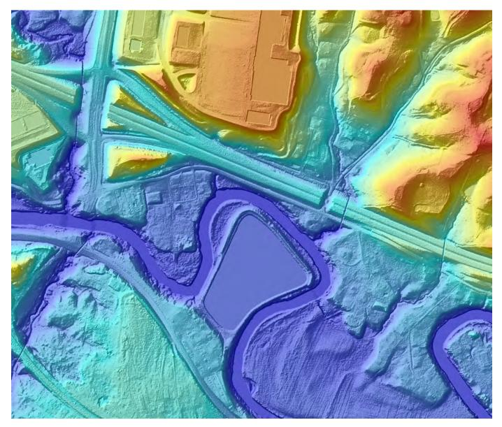
**Figure 12.** Colorized version of the hydro-enforced digital elevation model. This is the same surface shown in figure 11, with the breaklines removed for clearer depiction of the hydro-enforcement modifications to the surface. Light detection and ranging data courtesy of Cabell County, West Virginia, 2009. Digital elevation model developed from light detection and ranging data by the Earth Resource Observation and Science Center, 2010.
