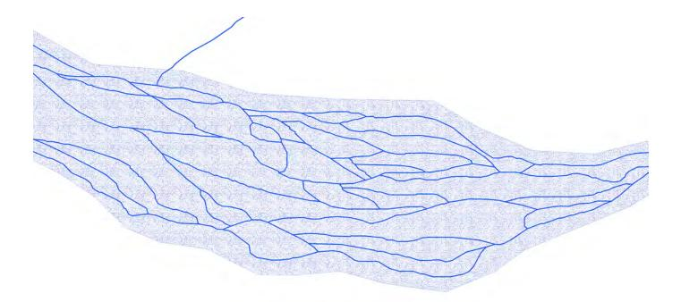
**Figure 20.** Example of a braided stream area (EType 1402). Shown as the light blue background polygon, this feature defines an area dense with stream braids depicted in darker blue lines. There are no explicit rules for how this polygon should be delineated; the data producer is to exercise their best professional judgement. This feature is for elevation reference. It is not used in the National Hydrography Dataset and has no National Hydrography Dataset equivalent.
