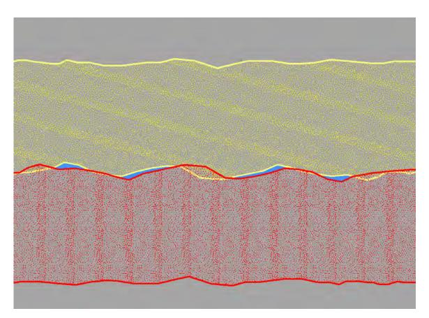
**Figure 1.** Single coverage collection, no overlap. Adjacent swaths (red and yellow) in this example have been collected with insufficient overlap, causing gaps in coverage. The blue areas depict data voids, which are grounds for rejection of the project.
