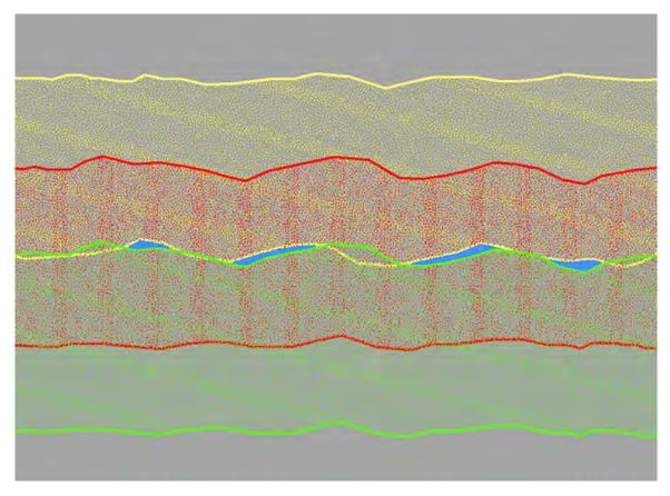
**Figure 2.** Designed double coverage collection, 50-percent overlap. In this example, three adjacent overlapping swaths (green, red, and yellow) have been collected. Because the design of the project achieved the required aggregate nominal pulse density (ANPD) through double-coverage, the blue areas that are not covered by two swaths are considered data voids, which are grounds for rejection of the project.
