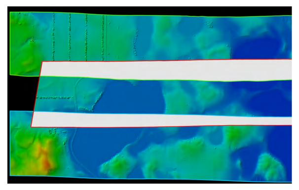
**Figure 4.** Graphic depiction of swath overlap. Three light detection and ranging swaths are depicted with the edges colored blue, red, and green. Each adjacent pair of swaths shares one overlap region shown in gray.
