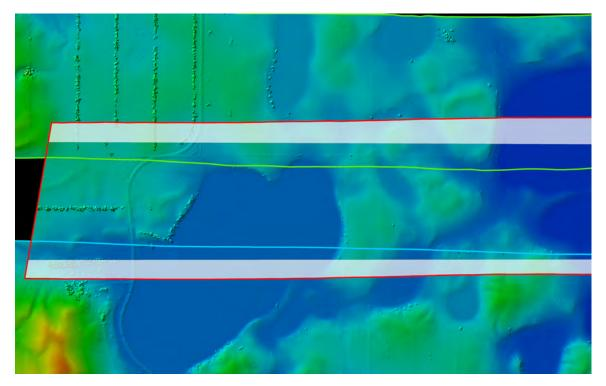
**Figure 5.** Graphic depiction of swath overage. Three light detection and ranging swaths are depicted with the edges colored blue, red, and green. Each individual swath has an overage region shown in gray for each adjacent, overlapping swath.
