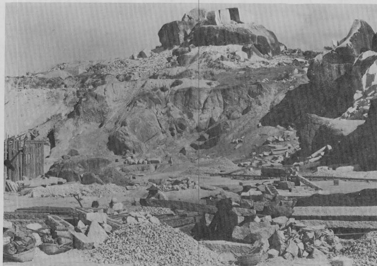
15. Granite quarry near Ssu-ming (Terrain Unit III). Knobs are fresh rock suitable for dimension stone and road metal; intervening areas underlain by deeply decayed bedrock. (Copyright, Nat. Geog. Soc., 1932, 75956-A).
