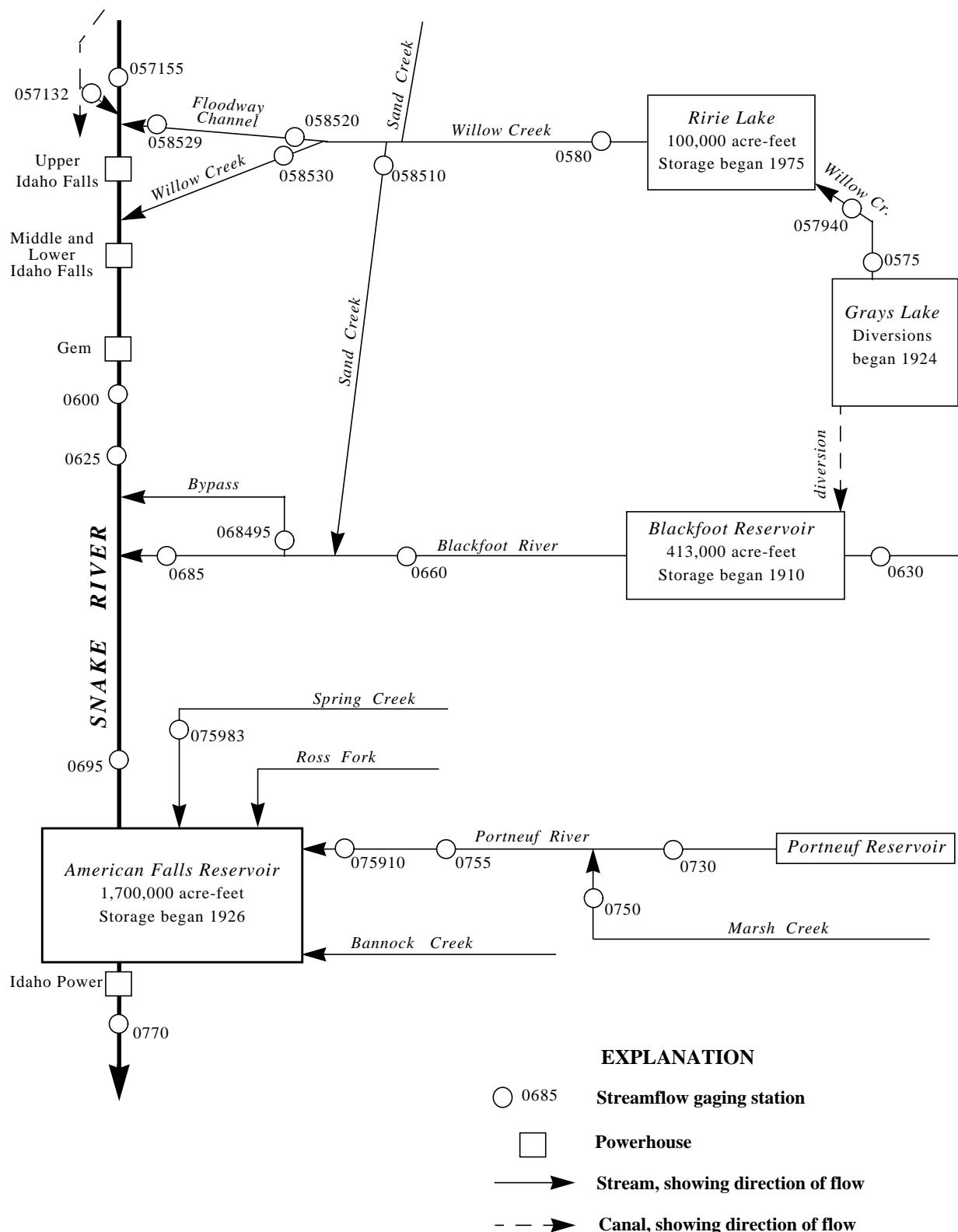
**Figure 18.** Schematic diagram showing gaging stations in Snake River Basin between Idaho Falls and Snake River at Neeley.
