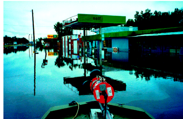
Neuse River flooding in Goldsboro, N.C. Acoustic Doppler current profiler used for discharge measurements shown in the foreground on the boat bow.
