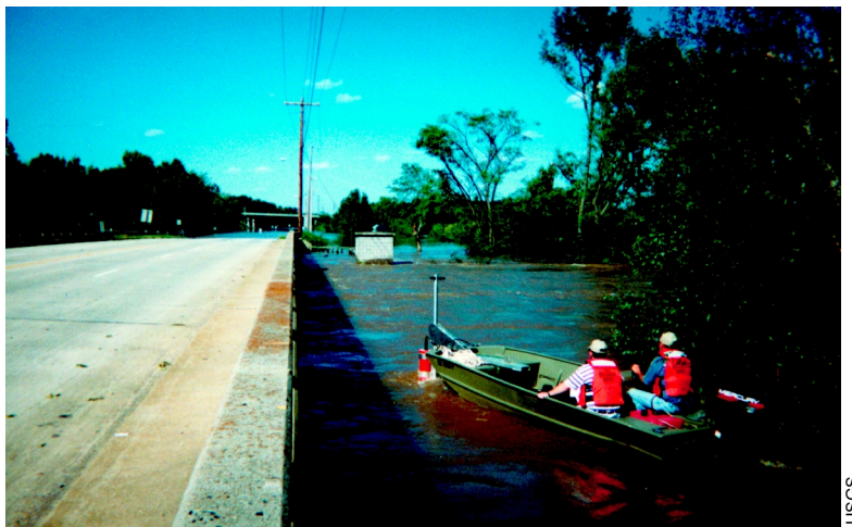
USGS staff making a discharge measurement using an acoustic Doppler current profiler on the Tar River
