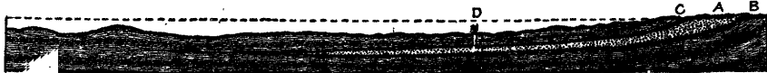
FIG. 3.—Ideal section illustrating the thinning out of a porous water-bearing bed, A, inclosed between impervious beds, B and C, thus furnishing the necessary conditions for an artesian fountain, D. (After T. C. Chamberlin.)
