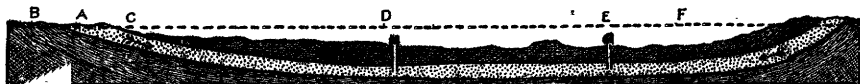
FIG. 2.—Ideal section illustrating the chief conditions of artesian wells. A, a porous stratum; B and C, impervious beds below and above A, acting as confining strata; F, the height of the water level, "artesian head," in the porous bed A, or, in other words, the height of the reservoir or fountain head; D and E, flowing wells springing from the porous water-filled bed A. (After T. C. Chamberlin.)
