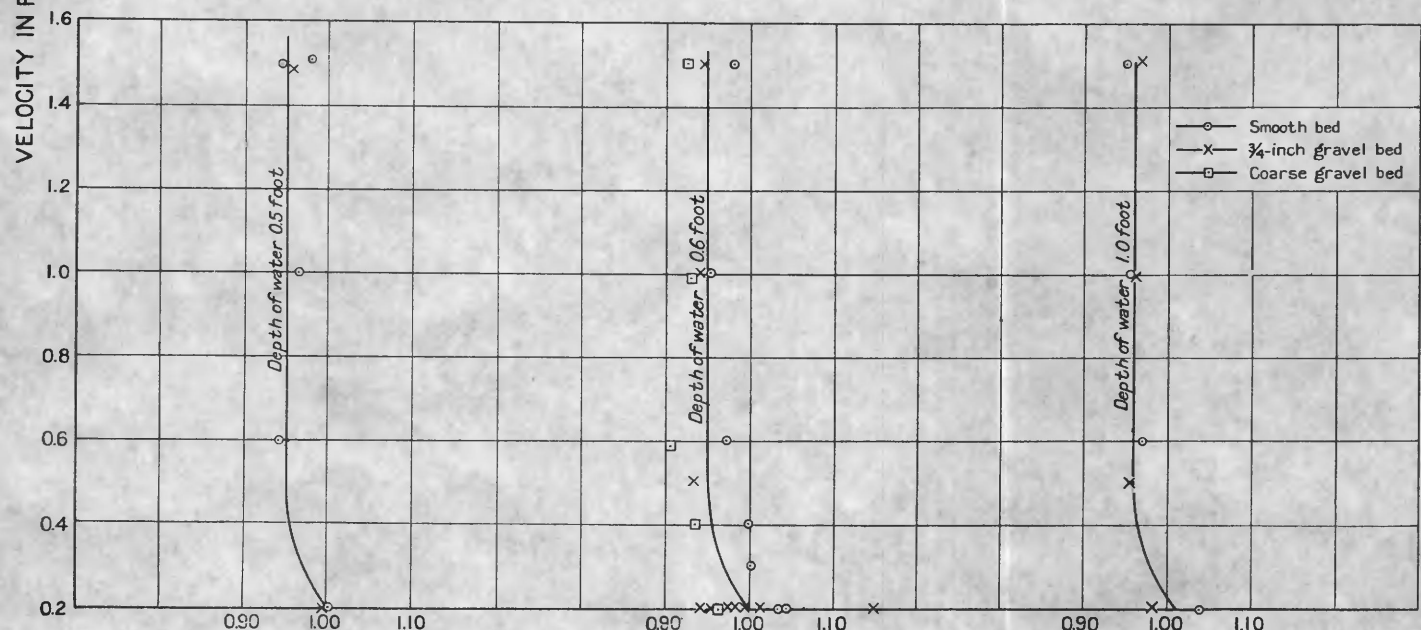
VARIATION OF COEFFICIENTS WITH CHANGE IN VELOCITY, 0.5-DEPTH METHOD, PYGMY CURRENT METERS.
