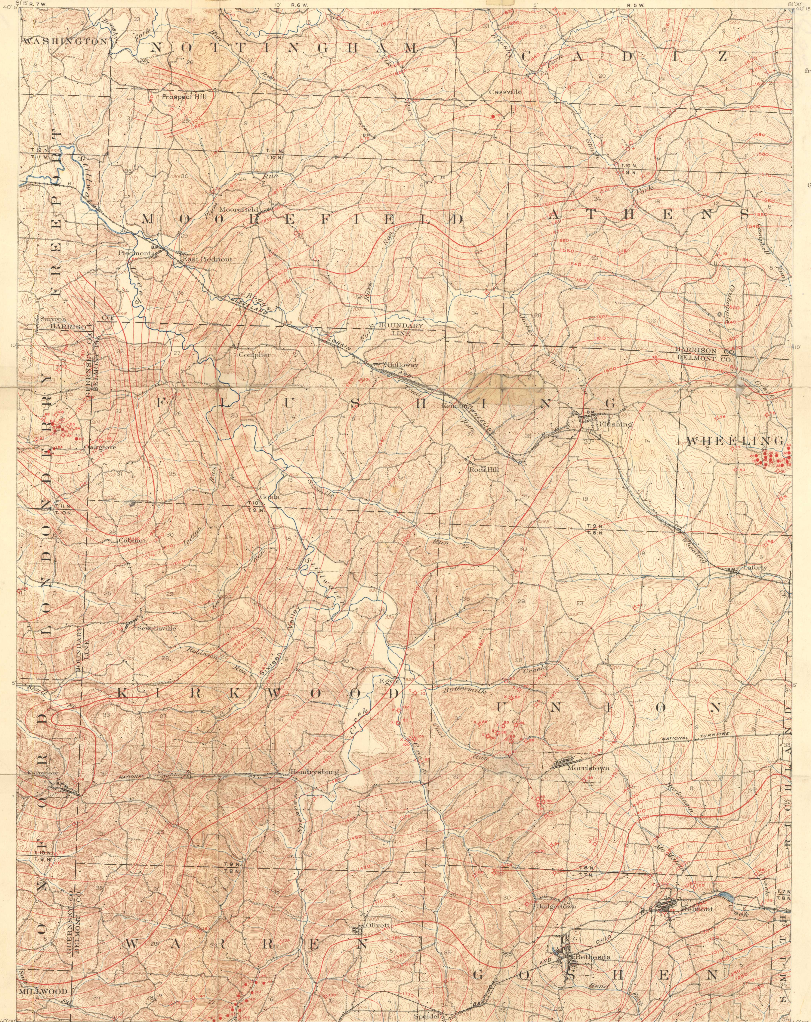
MAP OF FLUSHING QUADRANGLE, OHIO, SHOWING CONTOURS ON TOP OF BEREA SAND
