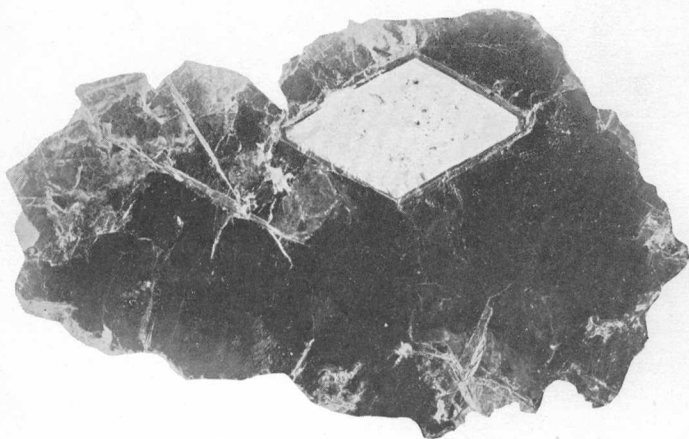
C. SHEET OF BIOTITE FROM MITCHELL COUNTY, N. C., INCLOSING A RHOMBIC CRYSTAL OF MUSCOVITE, BOTH HAVING THE SAME CLEAVAGE PLANES.
