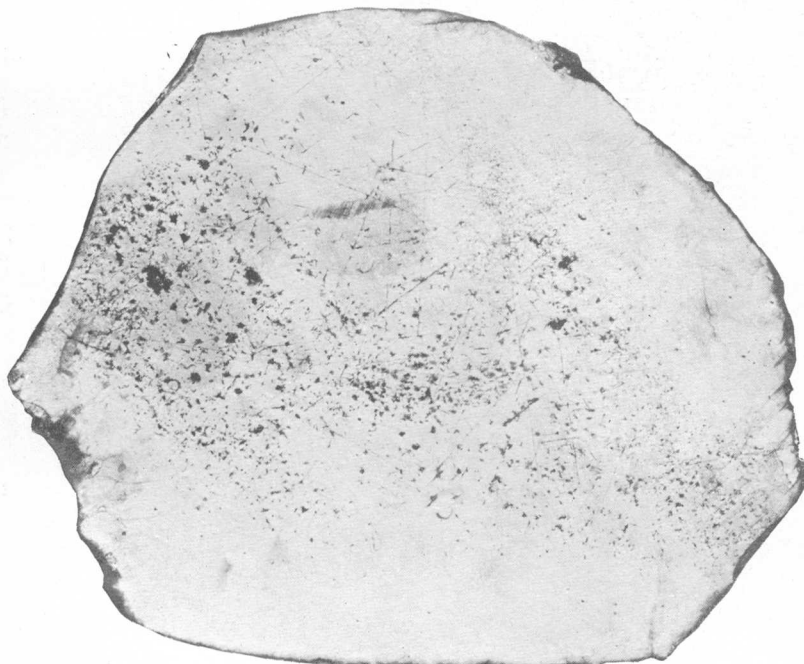
B. MICA SLIGHTLY "SPECKED" WITH MAGNETITE.
