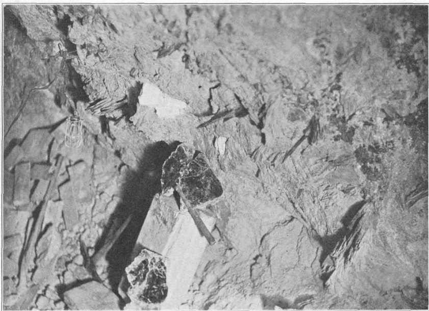
B. CRYSTALS OF MICA IN PEGMATITE AND BLASTED LOOSE ON 200-FOOT LEVEL OF NEW YORK MICA MINE, NEAR CUSTER, S. DAK.
