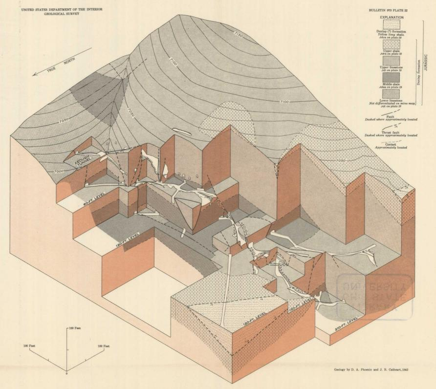
ISOMETRIC BLOCK DIAGRAM OF THE MINA DEVELOPMENT COMPANY MINE AND VICINITY
