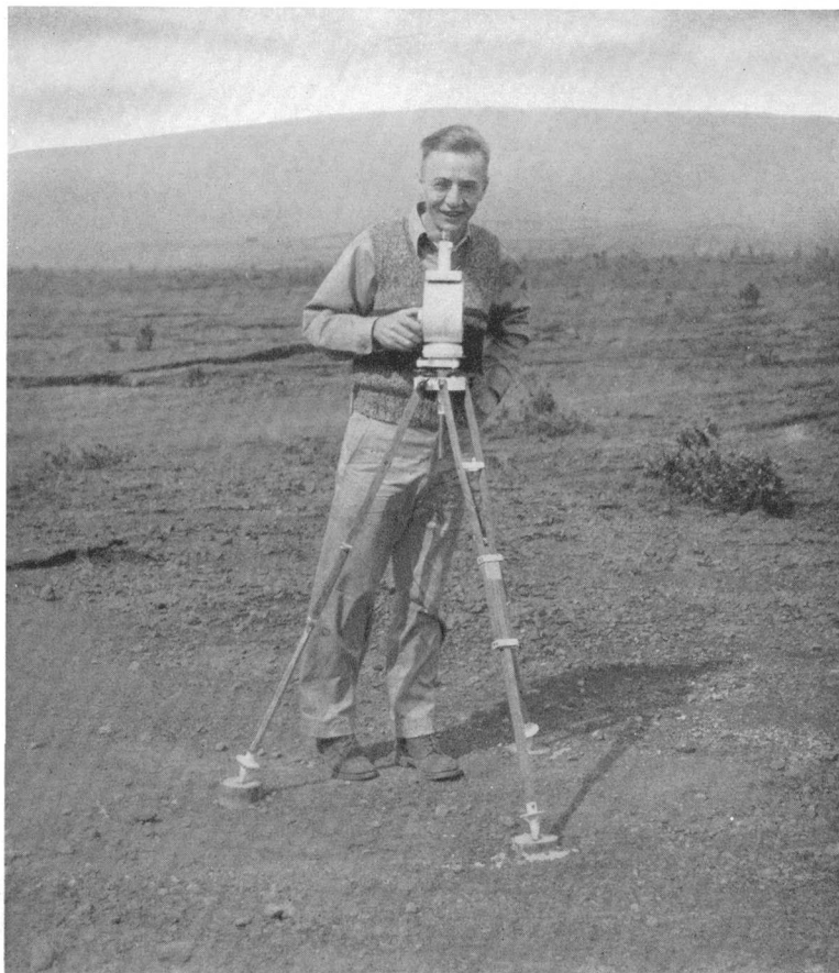
FIGURE 36.—Magnetometer set up for observations on one of the permanent stations. Concrete cups for tripod legs facilitates achieving the same position of the instrument at each reoccupation.
