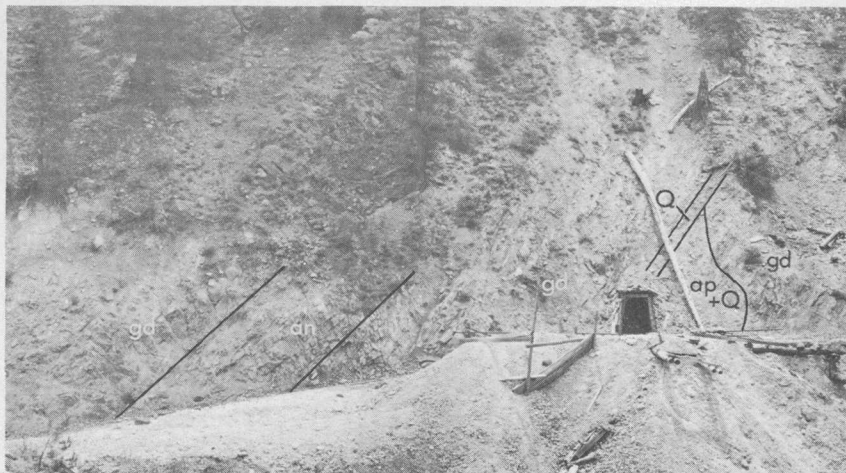
FIGURE 17.—Main adit portal and dump, Little Queens mine. The adit was driven along a quartz vein (Q) in granodiorite (gd) country rock. Aplite (ap) occurs locally. About 60 feet to the left of the portal is an andesite dike (an), which trends more or less parallel to the vein.
