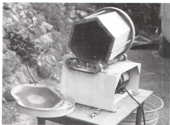
Figure 1. The 40-lb, 4-gal tumbler with 1/3-hp electric motor used in this study. Metal end and rubber gasket have been removed, showing hexagonal shape and rubber liner, having 78-cm internal circumference.
