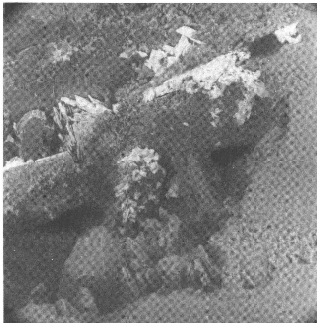
Figure 7. Scanning electron microscope backscattered-electron image of REE minerals (bright) and quartz crystals (dark) around a "thunder egg" vug. Field of view is approximately 0.7 mm.
