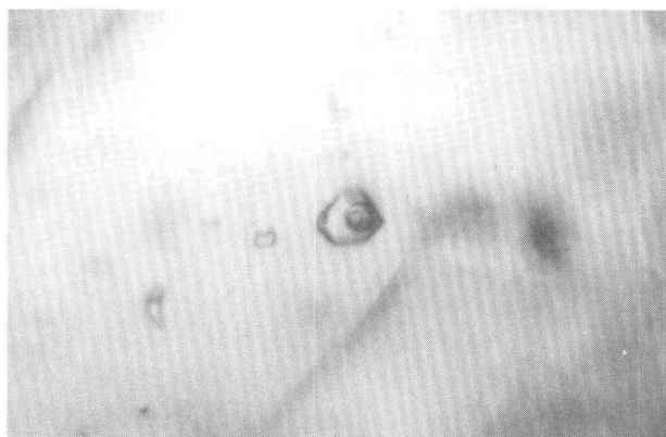
Figure 2. Typical type I inclusion from Little Creek prospect, showing three phases at -10^\circ\text{C} . Type I inclusions contain 90–92 mole percent H 2 O, 6–8 mole percent CO 2 , 1 mole percent CH 4 , and <1 mole percent N 2 . Inclusion is 10 \mu\text{m} in diameter.
