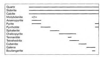
**Figure 9.** General paragenetic sequence for hypogene minerals in the Carrietown mineralized area, Idaho. Lines represent periods of deposition; time progressing to the right.
