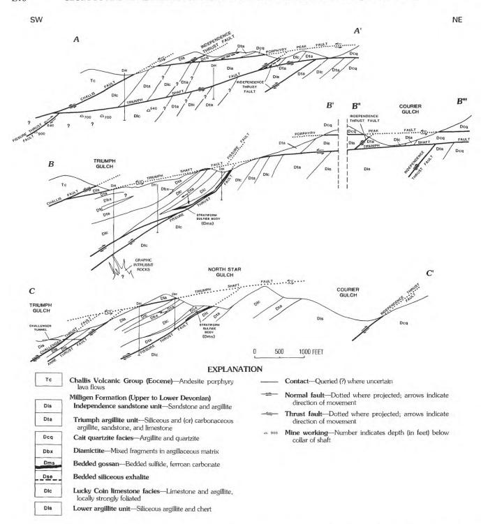
**Figure 4.** Structural cross sections, Triumph mine area, Idaho. Lines of section are shown in figure 3. *A–A'*, North of Triumph mine (Independence mine area). *B–B'*, *B''–B'''*, Across the northern part of Triumph mine (Triumph shaft area). *C–C'*, Through the southern Triumph mine (North Star mine area).
