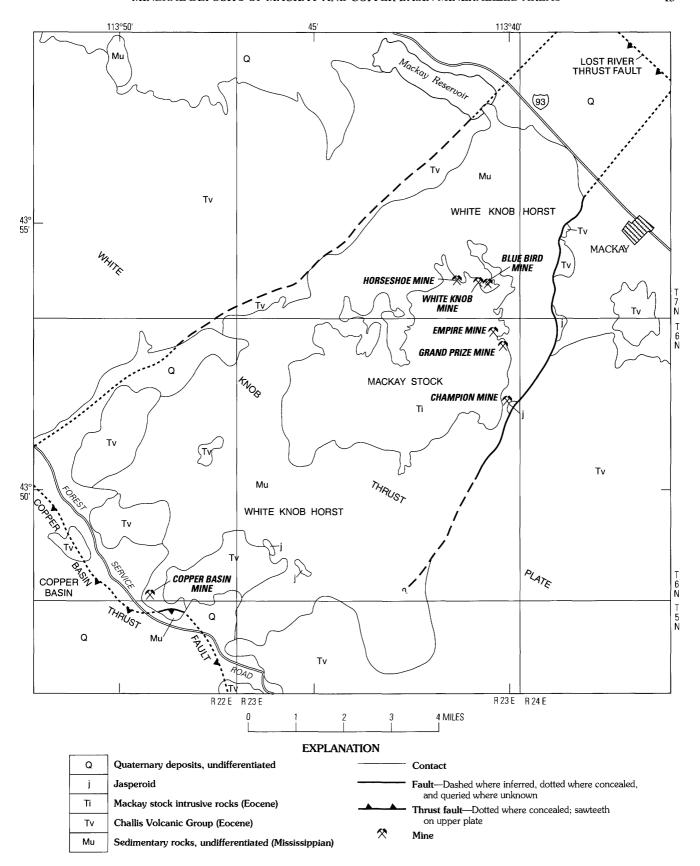
**Figure 2.** Map showing simplified geology, structural elements, and location of mines, Mackay and Copper Basin mineralized areas, White Knob Mountains, Idaho. Geology modified from Nelson and Ross (1968, 1969a) and Dover (1981).
