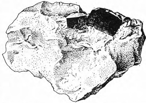
FIG. 18.—Disseminated galena in oil rock from the Enterprise mine, Platteville, Wis.
