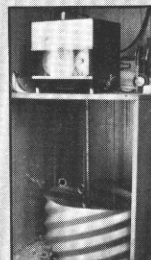
Digital Water Level Recorder
