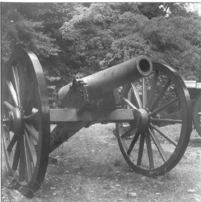
Figure 5. Cast bronze "Light" 12-pounder gun-howitzer, or Napoleon, at Howison's Hill. This gun was made in 1864 by James R. Anderson and Co., Tredegar Foundry, Richmond, Va. (Hazlett and others, 1988). Although cast long after the battle, this gun is virtually identical to Napoleons that would have been used during the Battle of Fredericksburg.
