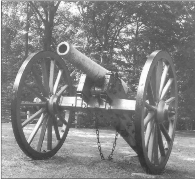
Figure 9. Cast bronze 14-pounder (3.8-in) James rifle at Prospect Hill. This gun was made in 1861 by Ames Co., Chicopee, Mass. (Hazlett and others, 1988).
